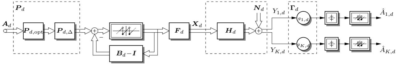
Fig. 1. Block diagram of sorted Tomlinson-Harashima precoding.
