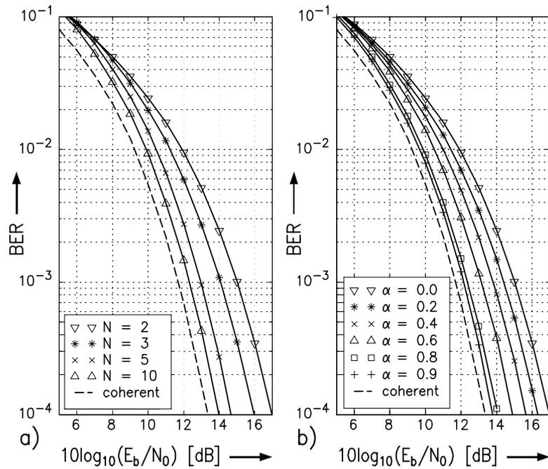
Figure 3: BER vs.  $10 \log_{10}(E_b/N_0)$  for the noncoherent receiver with a) nonrecursively and b) recursively generated reference symbol  $q_{\text{ref}}[k-1]$ . For comparison the BER for a coherent receiver is also shown.
