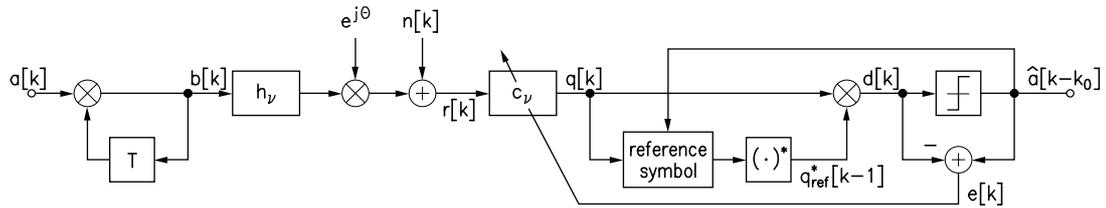
Figure 1: Block diagram of the discrete-time transmission model under consideration with linear equalization combined with noncoherent DF-DD.
