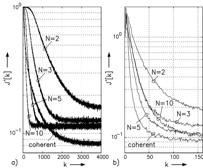
Figure 2: Learning curves for a) modified LMS and conventional (coherent) LMS algorithm; b) modified RLS and conventional (coherent) RLS algorithm.
