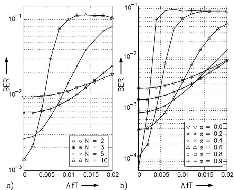
Figure 4: BER vs.  $\Delta f T$  for the noncoherent receiver with a) nonrecursively ( $10 \log_{10}(E_b/N_0) = 12$  dB) and b) recursively ( $10 \log_{10}(E_b/N_0) = 14$  dB) generated reference symbol  $q_{\text{ref}}[k-1]$ .
