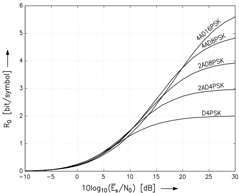
**Figure 2:** Cutoff rate  $R_0$  vs.  $\bar{E}_s/N_0$ . Non-coherent ADPSK and BICM over Rayleigh fading.
