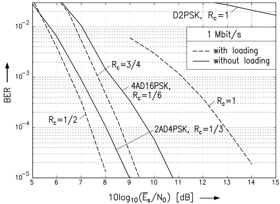
**Figure 5:** BER vs.  $\bar{E}_s/N_0$  for adaptive and non-adaptive coded OFDM with non-coherent ADPSK over power lines. Data rate  $R_T = 1$  Mbit/s.
