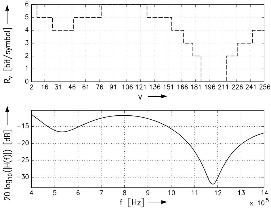
**Figure 3:** Top: Assignment of rates  $R_v$  to subcarrier  $v$  with loading algorithm by Piazza [16].  $R_T = 2$  Mbit/s,  $BER_T = 10^{-3}$ ,  $R_c = 1/2$ . Bottom: Power-line channel amplitude transfer function  $|H(f)|$  according to [3].
