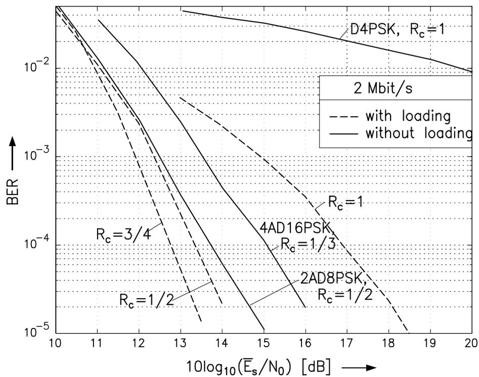
**Figure 6:** BER vs.  $\bar{E}_s/N_0$  for adaptive and non-adaptive coded OFDM with non-coherent ADPSK over power lines. Data rate  $R_T = 2$  Mbit/s.
