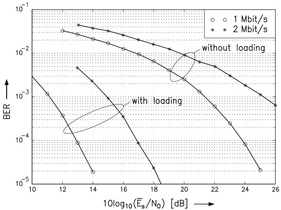
**Figure 4:** BER vs.  $\bar{E}_s/N_0$  for adaptive and non-adaptive uncoded OFDM with non-coherent ADPSK over power lines.
