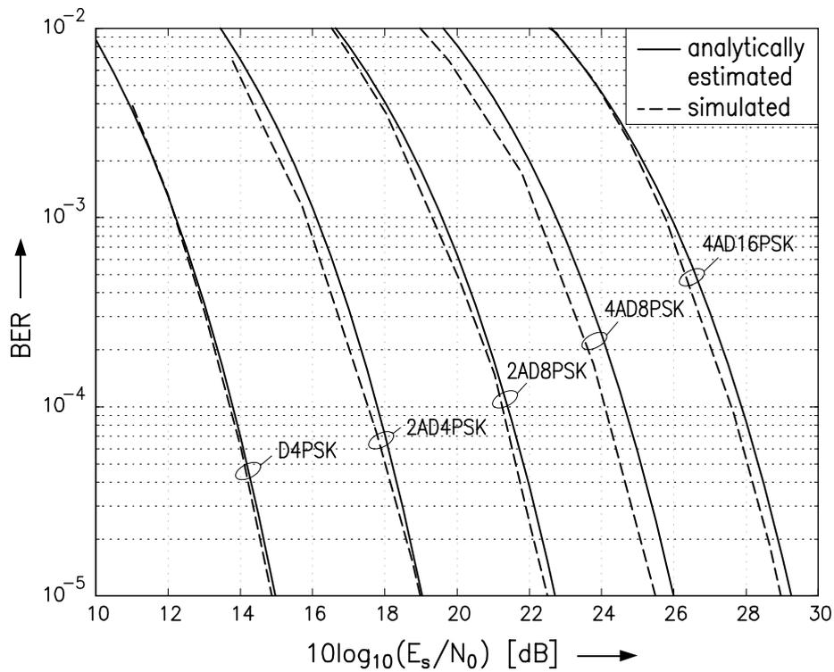
**Figure 1:** BER vs.  $E_s/N_0$  of ADPSK over AWGN channel. Solid lines: analytical approximation. Dashed lines: simulation. From left to right: D4PSK, 2AD4PSK  $\rho = 1.1$ , 2AD8PSK  $\rho = 0.6$ , 4AD8PSK  $\rho = 0.6$ , 4AD16PSK  $\rho = 0.3$ .
