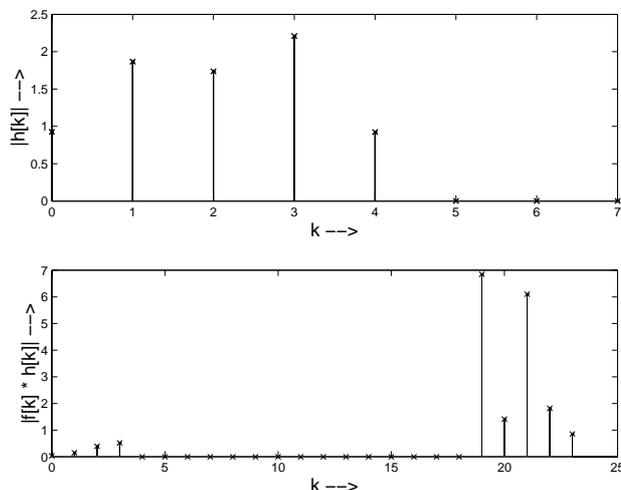
Figure 5: Magnitude of original and transformed impulse response (channel 2).
