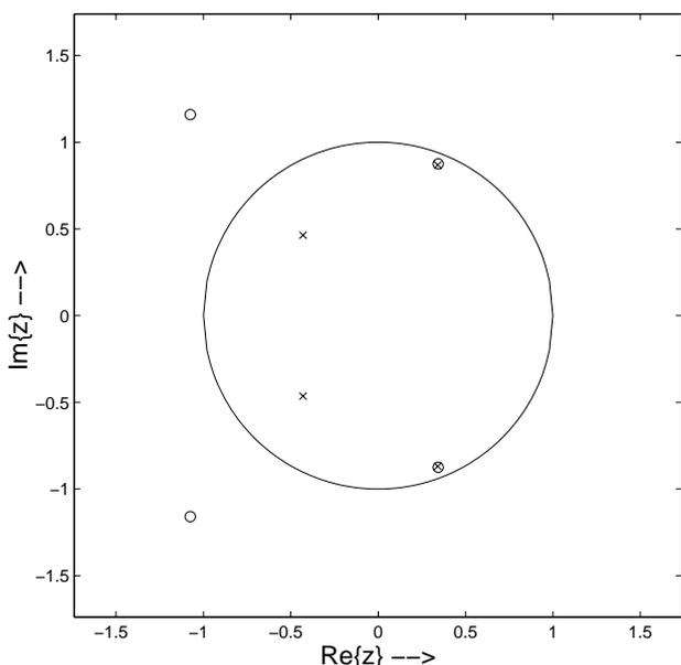
Figure 3: Zeros of  $H(z)$  ('o') and zeros of overall transfer function including prefilter ('x') (channel 1).
