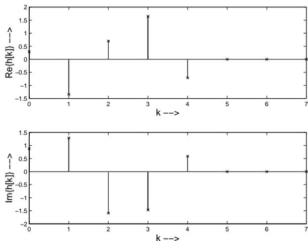
Figure 4: Real and imaginary part of impulse response of channel 2.
