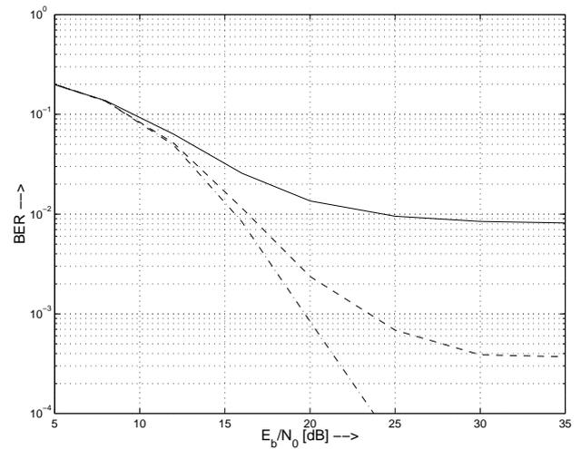
Figure 8: BER at equalizer output vs.  $E_b/N_0$  for EDGE transmission over EQ50 channel. Equalization: RSSE ( $Z = 2$ ) with proposed prefiltering method using filters with different orders. Solid line:  $q_f = 15$ , dashed line:  $q_f = 22$ , dash-dotted line:  $q_f = 32$ .
