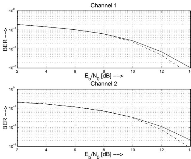
Figure 7: BER vs.  $E_b/N_0$  for RSSE ( $Z = 2$ ) with proposed prefiltering method (solid lines) and allpass prefiltering (dashed lines). Top: channel 1, bottom: channel 2.
