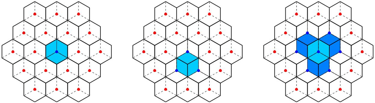
Fig. 3. Hexagonal grid structure of the scenario with cooperation at a single BS (left), with cooperation of three sectors of three BSs (center), and cooperation of nine sectors of seven BSs (right). Situation shown for 3-tier cluster with one central BS, 6 BSs at first tier, and 12 BSs at second tier ( $N_{\text{total}} = 37$ ). Area of UEs included in coordination in shades of blue; identical characteristics indicated by equal shades.
