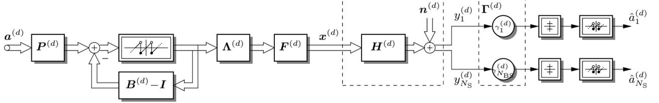
Fig. 2. Block diagram of Tomlinson-Harashima precoding. Situation shown for  $d$ -th carrier of MIMO OFDM system.
