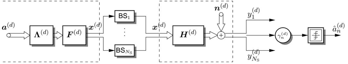
Fig. 1. Block diagram of (zero-forcing) linear pre-equalization. Situation shown for  $d$ -th carrier of MIMO OFDM system.
