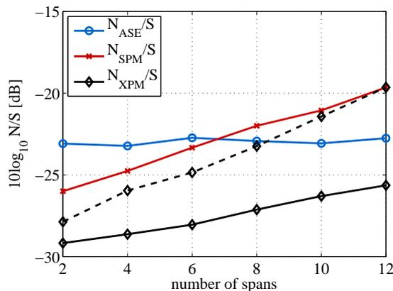
Fig. 2. Separated noise powers versus distance; launch power per channel: -6 dBm, 3 WDM channels; dashed line: Non-linear crosstalk for the setup with 9 WDM channels.
