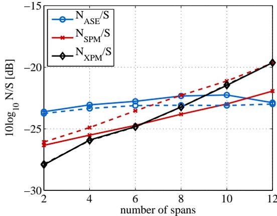
Fig. 7. Separated noise powers versus distance; 9 WDM channels (-6 dBm); dashed lines: no SPM compensation; solid lines: with SPM,  $L_{\text{eff,RX}} = 6$  km.
