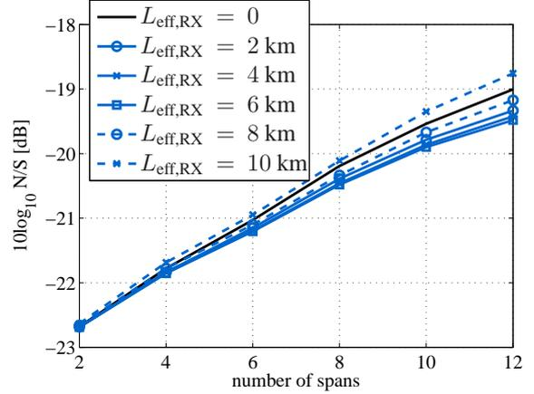
Fig. 5. Estimated  $N/S$  versus transmission distance for different settings of the non-linear phase modulator.
