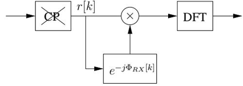
Fig. 4. Non-linear phase-shifting at the OFDM receiver.
