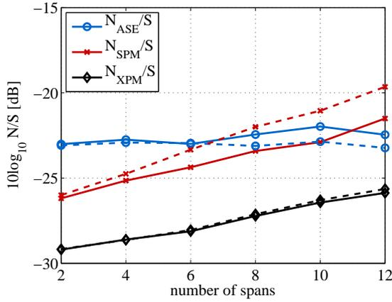
Fig. 6. Separated noise powers versus distance; 3 WDM channels (-6 dBm); dashed lines: no SPM compensation; solid lines: with SPM,  $L_{\text{eff,RX}} = 6$  km.
