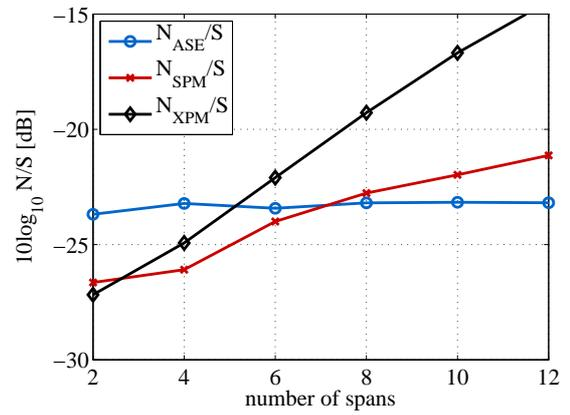
Fig. 3. Separated noise powers versus distance; launch power per channel: -6 dBm, 15 WDM channels.
