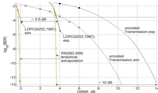
Fig. 6. Comparison of simulation (solid curves marked with right-pointing triangles and squares) and experimental results (solid curves marked with left-pointing triangles and circles) for OFDM channel model with (left curves) and without (right curves) soft-FEC. Maximum number of LDPC iterations: 10. Horizontal dashed line shows RS input BER for the output BER of  $10^{-13}$ .
