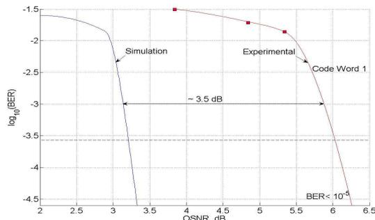
**Fig. 8.** 7% OH IRA-LDPC code is transmitted over the OFDM channel model. Simulation and experimental results for different IRA-LDPC code words reveal the maximal OSNR difference of 3.5 dB. Maximum number of IRA-LDPC iterations: 100. Horizontal line shows RS input BER for the output BER of  $10^{-5}$ .
