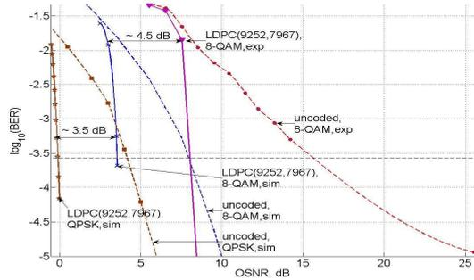
**Fig. 7.** Comparison of simulation and experimental (solid and dashed right curves) results for QPSK (solid and dashed left curves) and 8-QAM over OFDM channel model with (solid curves) and without (dashed curves) soft-FEC. Maximum number of LDPC iterations: 10.
