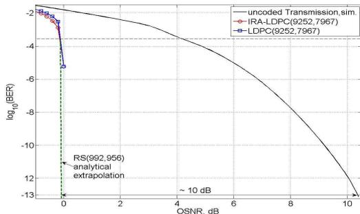
**Fig. 4.** OFDM channel model. 16% OH IRA-LDPC and standard irregular LDPC. Maximum number of LDPC iterations: 100. Horizontal line shows RS input BER for the output BER of  $10^{-13}$ .
