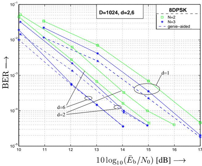
Fig. 6. BER over  $10 \log_{10}(\bar{E}_b/N_0)$ . OFDM with  $D = 1024$ , 8DPSK, and diversity  $d = 1, 2, 6$ . Conventional differential demodulation with  $N = 2$ . Iterative DF-DM with  $N = 3$  after four iterations.
