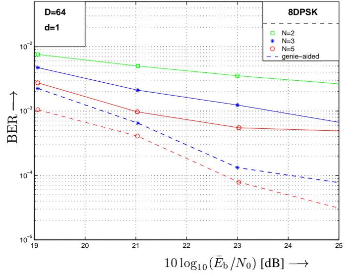
Fig. 7. BER over  $10 \log_{10}(\bar{E}_b/N_0)$ . OFDM with  $D = 64$ , 8DPSK, and diversity  $d = 1$  (independent processing of each OFDM symbol). Conventional differential demodulation with  $N = 2$ . Iterative DF-DM with  $N = 3, 5$  after four iterations.
