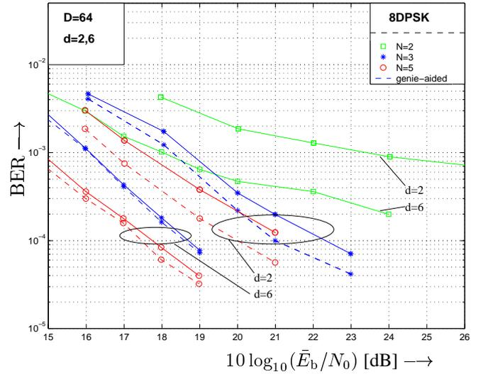
Fig. 8. BER over  $10 \log_{10}(\bar{E}_b/N_0)$ . OFDM with  $D = 64$ , 8DPSK, and diversity  $d = 2, 6$ . Conventional differential demodulation with  $N = 2$ . Iterative DF-DM with  $N = 3, 5$  after four iterations.
