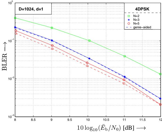
Fig. 5. BLER over  $10 \log_{10}(\bar{E}_b/N_0)$ . OFDM with  $D = 1024$ , 4DPSK, and diversity  $d = 1$  (independent processing of each OFDM symbol). Conventional differential demodulation with  $N = 2$ . Iterative DF-DM with  $N = 3, 5$  after four iterations.
