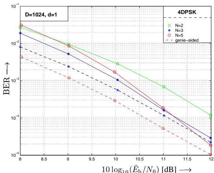
Fig. 3. BER over  $10 \log_{10}(\bar{E}_b/N_0)$ . OFDM with  $D = 1024$ , 4DPSK, and diversity  $d = 1$  (independent processing of each OFDM symbol). Conventional differential demodulation with  $N = 2$ . Iterative DF-DM with  $N = 3, 5$  after four iterations.
