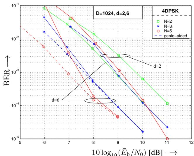
Fig. 4. BER over  $10 \log_{10}(\bar{E}_b/N_0)$ . OFDM with  $D = 1024$ , 4DPSK, and diversity  $d = 2, 6$ . Conventional differential demodulation with  $N = 2$ . Iterative DF-DM with  $N = 3, 5$  after four iterations.
