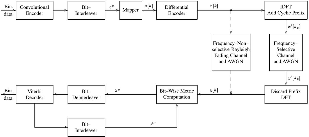
Fig. 1. Discrete-time system model.
