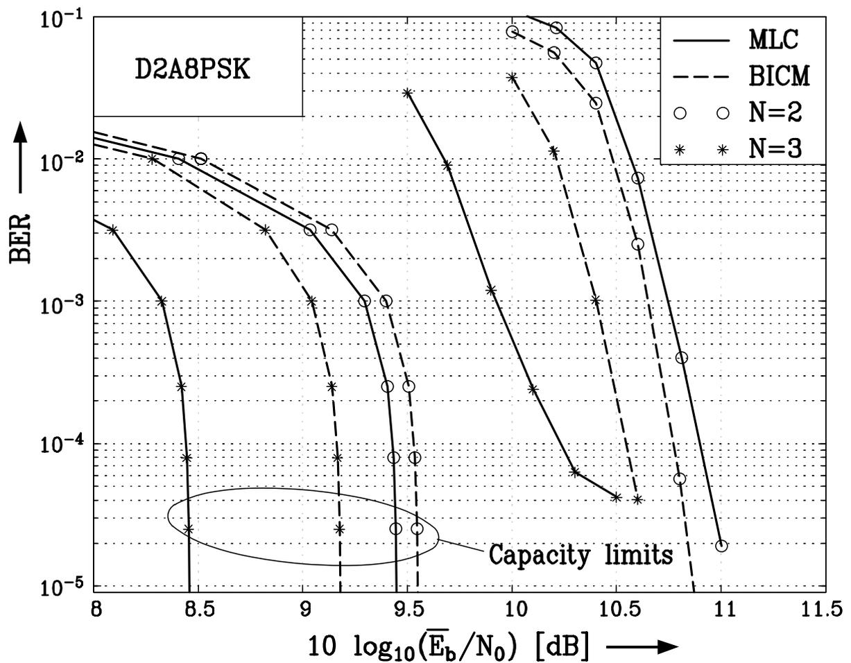
**Figure 8:** BER versus  $\bar{E}_b/N_0$  (in dB) for D2A8PSK ( $r_1/r_0 = 2.0$ ) with MLC (solid lines) and BICM (dashed lines). Rayleigh fading channel. Circles:  $N = 2$ , Stars:  $N = 3$ . Left hand side: respective rate–distortion capacity limits.
