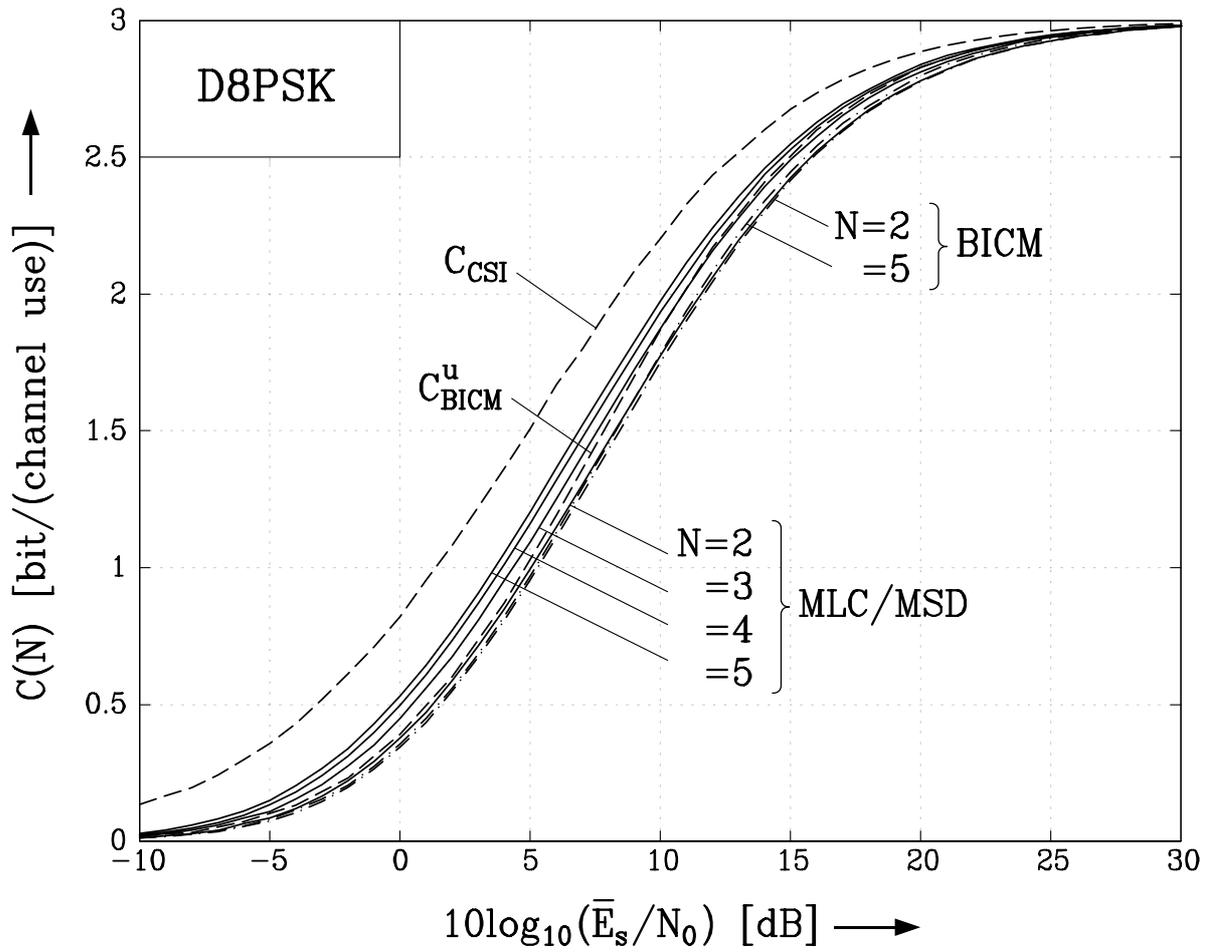
**Figure 4:** Normalized capacity for D8PSK. Solid lines: MLC with UL,  $N = 2, 3, 4, 5$  (from right to left). Dash-dotted lines: BICM with GL,  $N = 2, 5$  (from right to left). Rayleigh fading channel. Dashed Lines: Capacity  $C_{CSI}$  and bound  $C_{BICM}^u$ .
