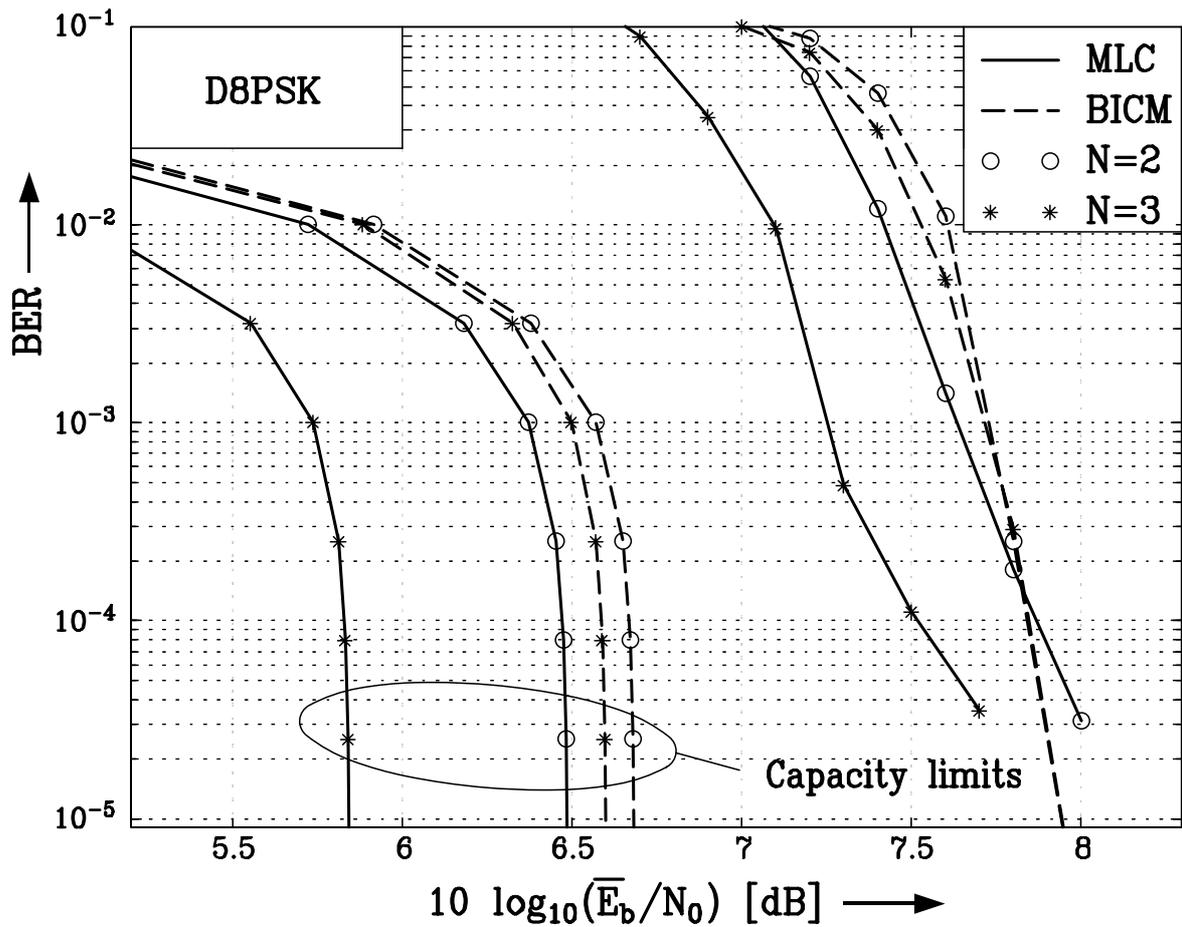
**Figure 7:** BER versus  $\bar{E}_b/N_0$  (in dB) for D8PSK with MLC (solid lines) and BICM (dashed lines). Rayleigh fading channel. Circles:  $N = 2$ , Stars:  $N = 3$ . Left hand side: respective rate-distortion capacity limits.
