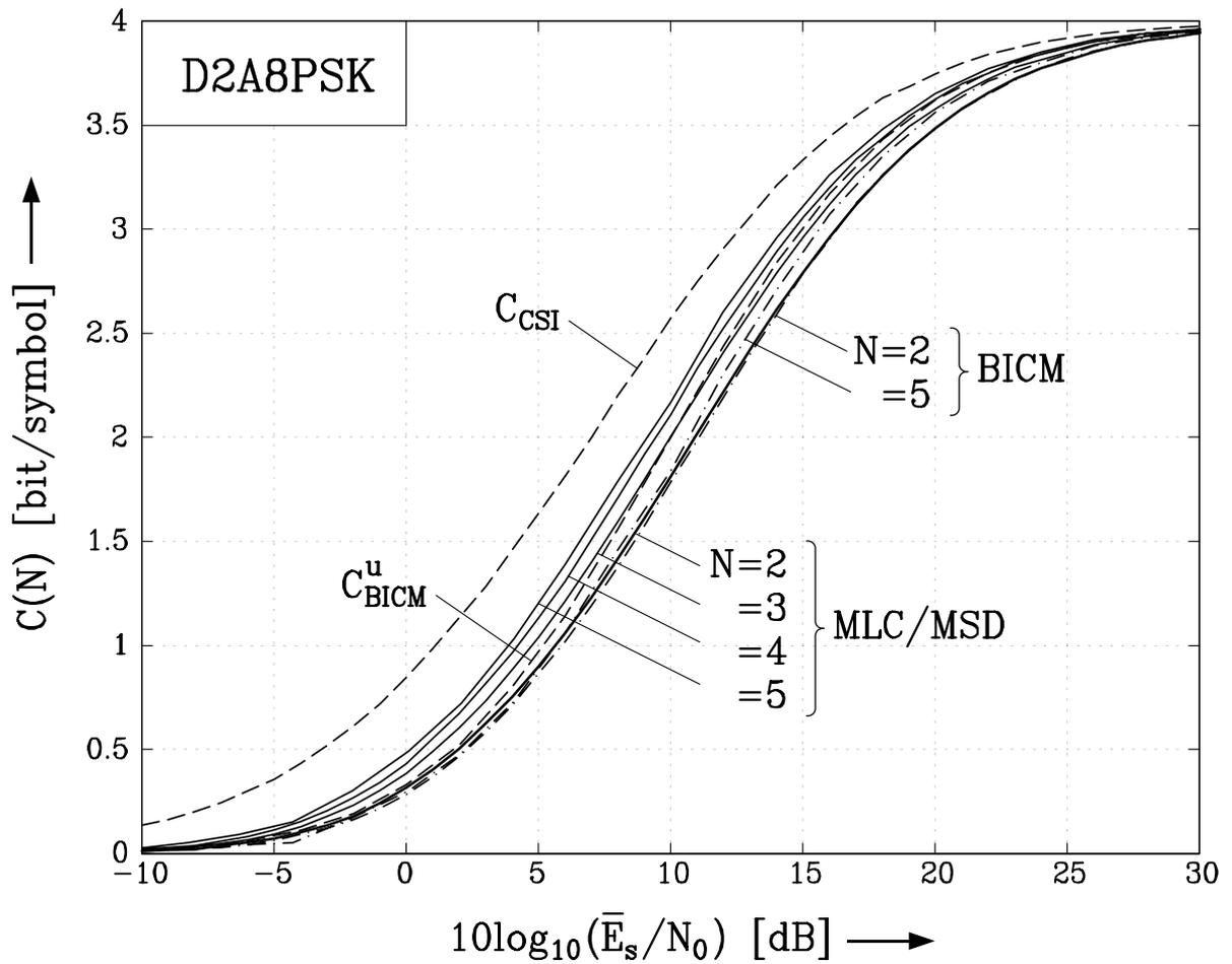
**Figure 6:** Normalized capacity for D2A8PSK with ring ratio  $r_1/r_0 = 2.0$ . Solid lines: MLC with UL,  $N = 2, 3, 4, 5$  (from right to left). Dash-dotted lines: BICM with GL,  $N = 2, 5$  (from right to left). Rayleigh fading channel. Dashed Lines: Capacity  $C_{CSI}$  and bound  $C_{BICM}^u$ .
