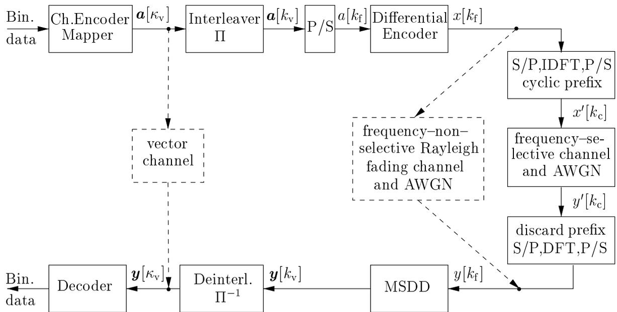
**Figure 1:** Discrete-time system model for OFDM transmission with differential encoding and the resulting equivalent fading channel and vector channel.
