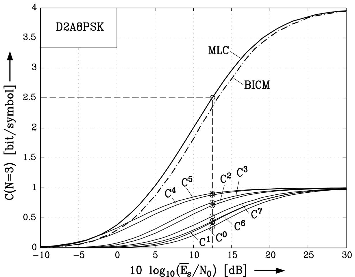
**Figure 5:** Capacity  $C(N = 3)$  and capacities  $C^0, \dots, C^7$  of the equivalent channels for D2A8PSK with ring ratio  $r_1/r_0 = 2.0$ . Solid lines: MLC with UL. Dash-dotted lines: BICM with GL. Rayleigh fading channel. Dashed lines: Rate design for  $C = 2.5$  bit/symbol.
