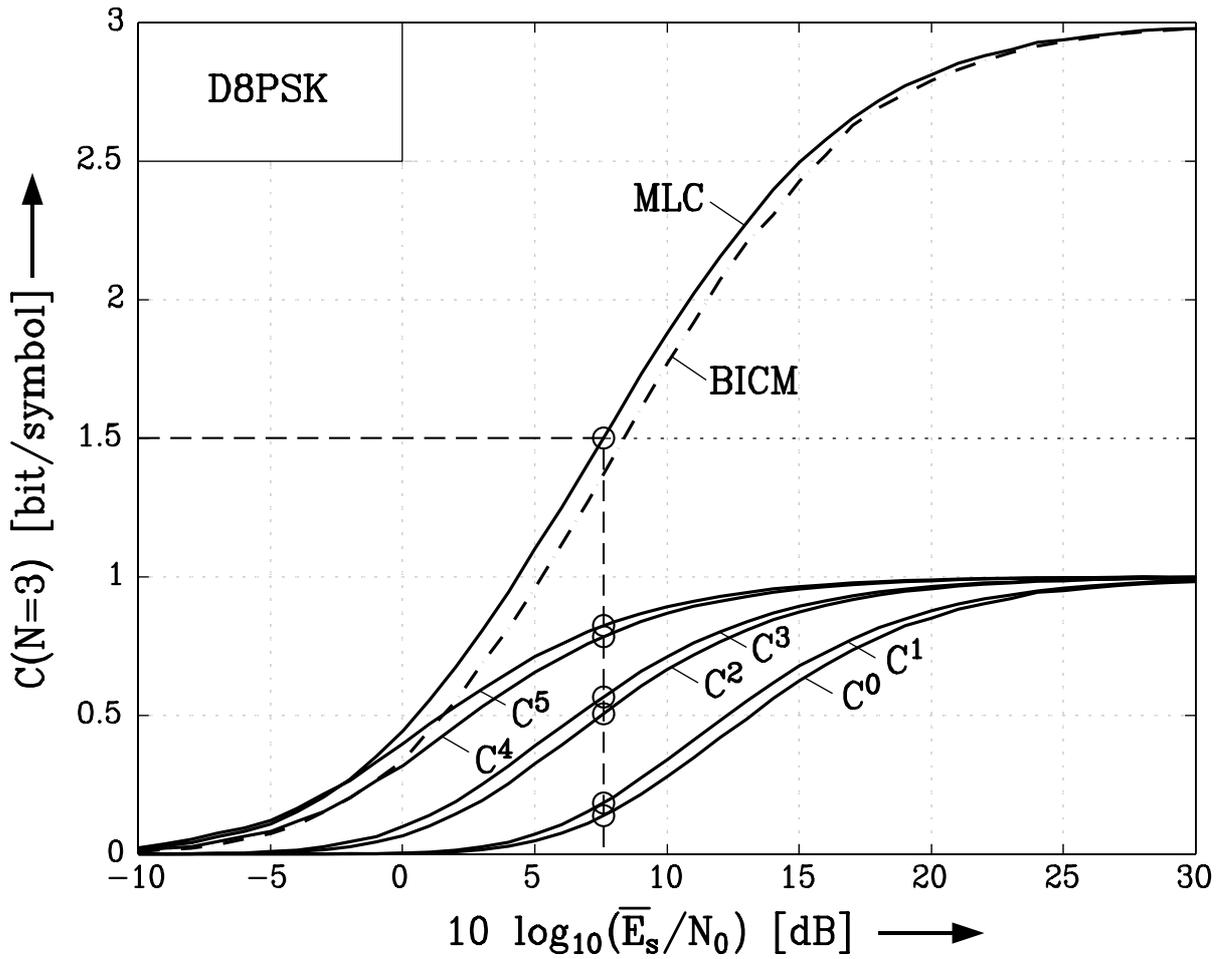
**Figure 3:** Capacity  $C(N = 3)$  and capacities  $C^0, \dots, C^5$  of the equivalent channels for D8PSK. Solid lines: MLC with UL. Dash-dotted lines: BICM with GL. Rayleigh fading channel. Dashed lines: Rate design for  $C = 1.5$  bit/symbol.
