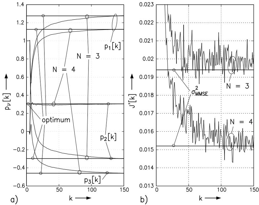
Figure 7: a) Predictor coefficients  $p_\nu[k]$ ,  $1 \leq \nu \leq N - 1$ , vs.  $k$  and b) learning curve (mean-squared error  $J'[k]$  vs.  $k$ ) of the adaptation algorithm for a Rayleigh fading channel ( $10 \log_{10}(E_b/N_0) = 20$  dB,  $B_f T = 0.03$ ,  $w = 0.99$ ). Predictors of order 2 ( $N = 3$ ) and 3 ( $N = 4$ ) are considered.
