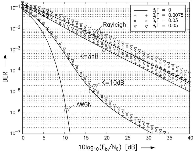
Figure 5: BER vs.  $10 \log_{10}(E_b/N_0)$  for QDPSK with genie-aided prediction-based DF-DD ( $N \rightarrow \infty$ ) for different fading bandwidths  $B_f$  and Ricean factors  $K$ . Jakes fading model is assumed.
