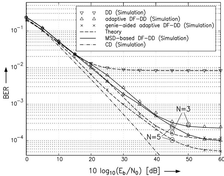
Figure 12: BER vs.  $10 \log_{10}(E_b/N_0)$  for QDPSK with conventional DD, adaptive prediction-based DF-DD ( $w = 0.99$ ), genie-aided adaptive (prediction-based) DF-DD ( $w = 0.99$ ), MSD-based DF-DD (here equivalent to prediction-based DF-DD with optimum fixed predictor coefficients), and CD for Rayleigh fading ( $B_f T = 0.03$ ). The theoretical BERs for conventional DD and genie-aided prediction-based DF-DD are also contained.
