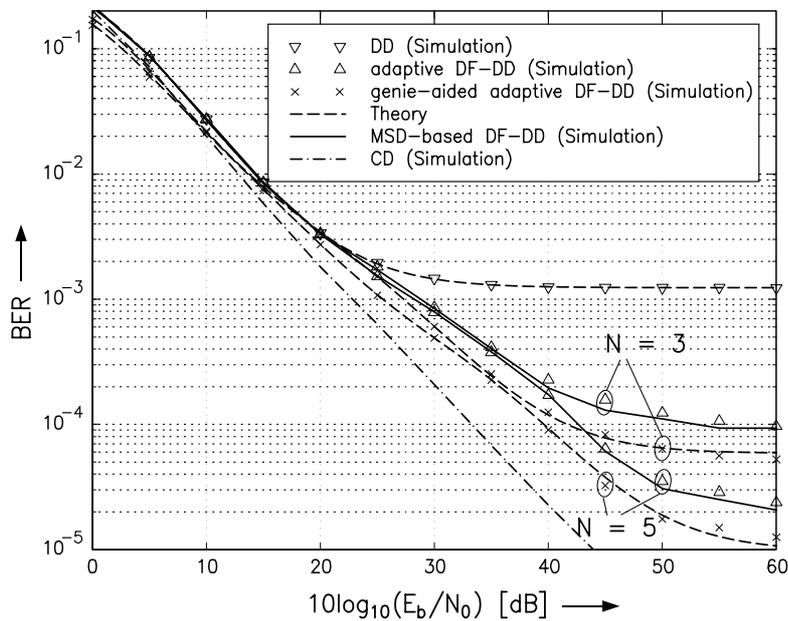
Figure 14: BER vs.  $10 \log_{10}(E_b/N_0)$  for QDPSK with conventional DD, adaptive (prediction-based) DF-DD ( $w = 0.99$ ), genie-aided adaptive DF-DD, MSD-based DF-DD, and CD for Ricean fading ( $10 \log_{10}(K) = 3$  dB,  $B_f T = 0.03$ ,  $f_D T = 0$ ). The theoretical BERs for conventional DD and genie-aided prediction-based DF-DD are also contained.
