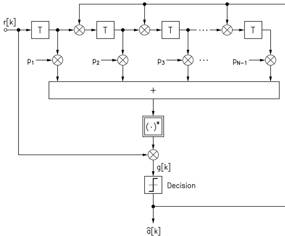
Figure 2: Structure of the prediction-based DF-DD receiver.
