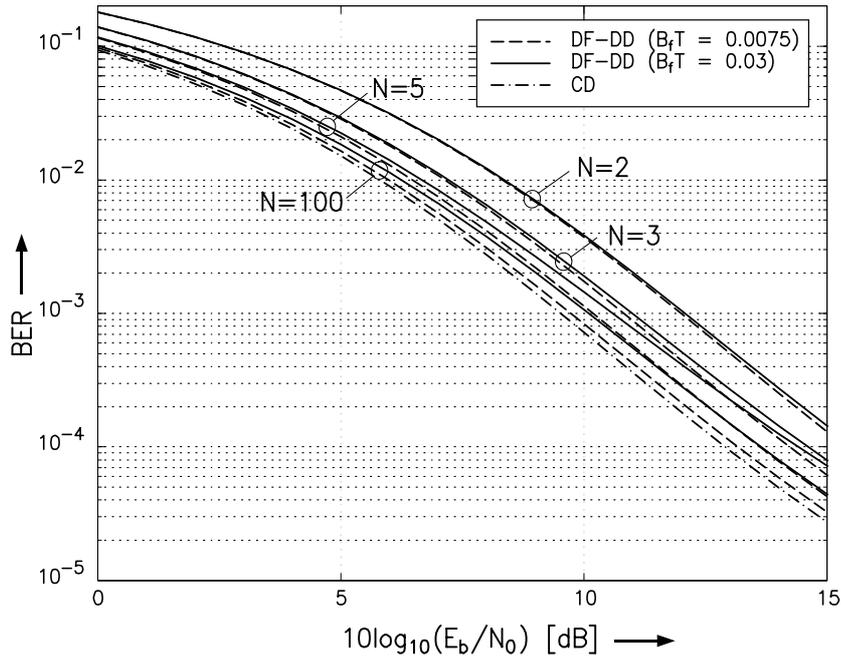
Figure 3: BER of coherent QPSK (denoted by ‘CD’) and QDPSK vs.  $10 \log_{10}(E_b/N_0)$  for conventional DD ( $N = 2$ ) and genie-aided prediction-based DF-DD ( $N = 3, 5, 100$ ) for Jakes fading model ( $10 \log(K) = 10$  dB,  $f_d T = 0$ ).
