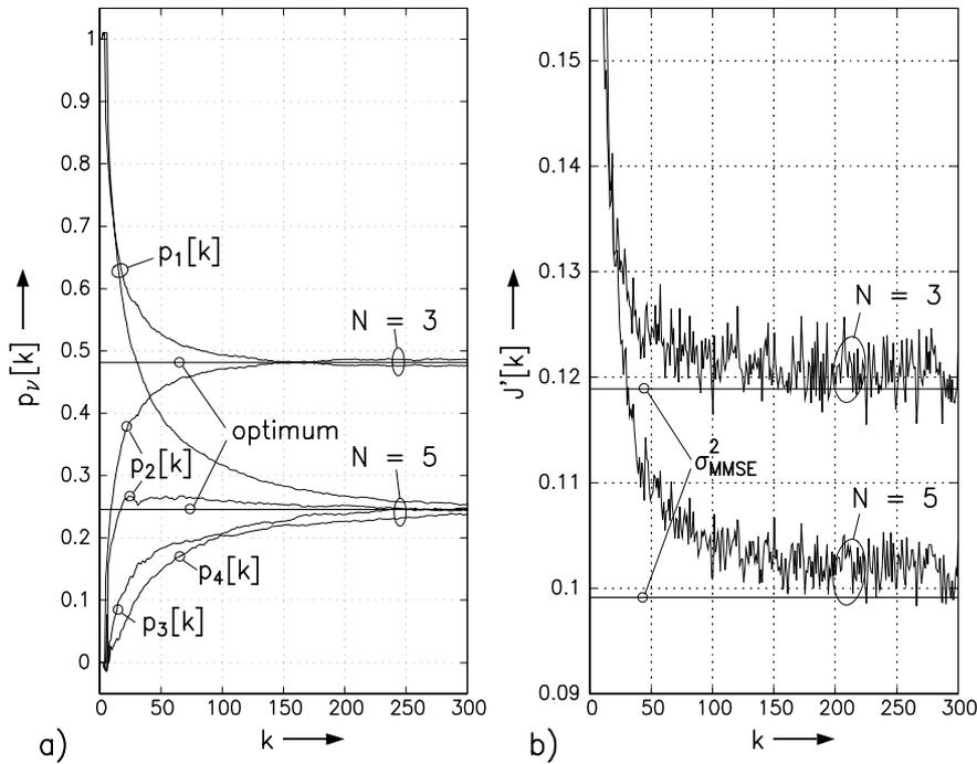
Figure 6: a) Predictor coefficients  $p_\nu[k]$ ,  $1 \leq \nu \leq N - 1$ , vs.  $k$  and b) learning curve (mean-squared error  $J'[k]$  vs.  $k$ ) of the adaptation algorithm for an AWGN channel ( $10 \log_{10}(E_b/N_0) = 8$  dB,  $w = 0.99$ ). Predictors of order 2 ( $N = 3$ ) and 4 ( $N = 5$ ) are considered.
