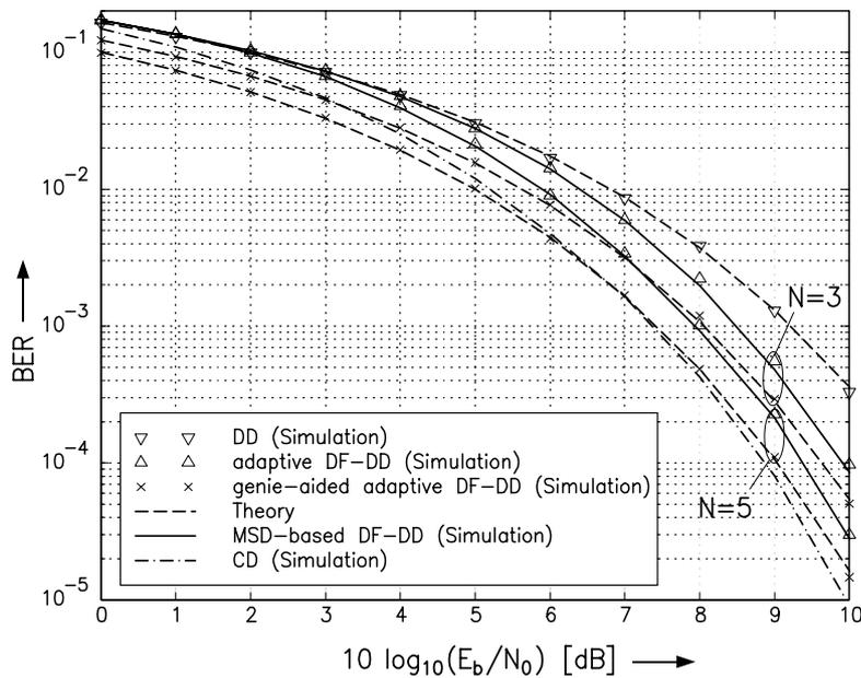
Figure 10: BER vs.  $10 \log_{10}(E_b/N_0)$  for QDPSK with conventional DD, adaptive prediction-based DF-DD ( $w = 1$ ), genie-aided adaptive (prediction-based) DF-DD ( $w = 1$ ), MSD-based DF-DD (here equivalent to prediction-based DF-DD with optimum fixed predictor coefficients), and CD for the AWGN channel. The theoretical BERs for conventional DD and genie-aided prediction-based DF-DD are also contained.
