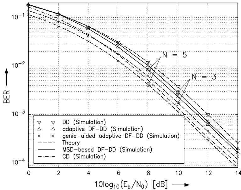
Figure 13: BER vs.  $10 \log_{10}(E_b/N_0)$  for QDPSK with conventional DD, adaptive (prediction-based) DF-DD ( $w = 0.99$ ), genie-aided adaptive DF-DD, MSD-based DF-DD, and CD for Ricean fading ( $10 \log_{10}(K) = 10$  dB,  $B_f T = 0.0075$ ,  $f_D T = 0$ ). The theoretical BERs for conventional DD and genie-aided prediction-based DF-DD are also contained.
