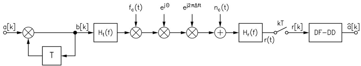
Figure 1: Block diagram of the transmission model.
