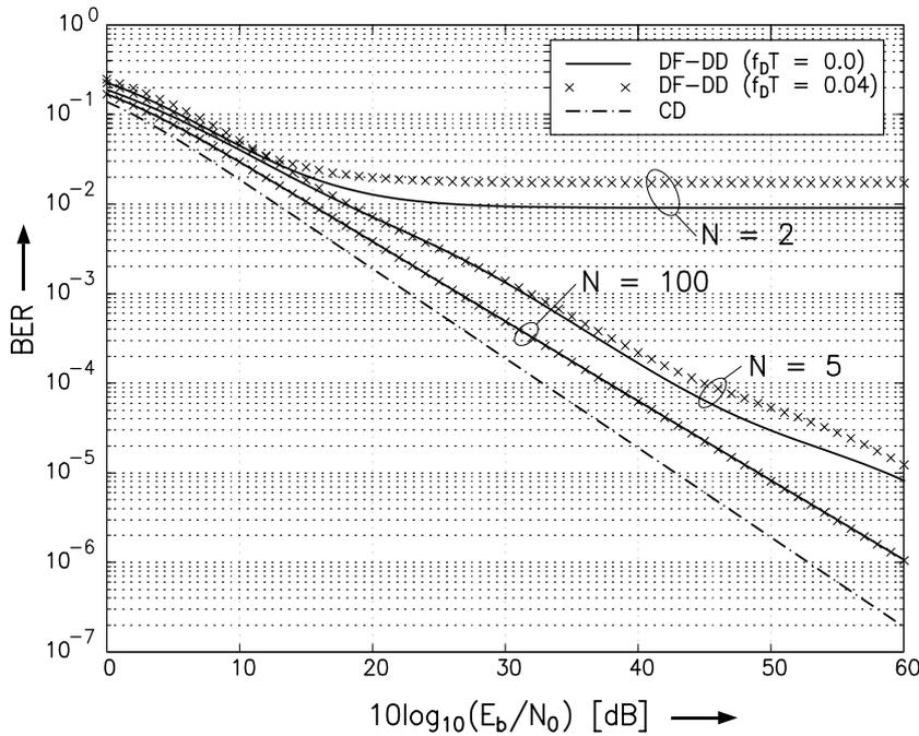
Figure 4: BER of coherent QPSK (denoted by ‘CD’) and QDPSK vs.  $10 \log_{10}(E_b/N_0)$  for genie-aided prediction-based DF-DD ( $N = 2, 5, 100$ ) for Jakes fading model ( $10 \log(K) = 3$  dB,  $B_f T = 0.05$ ).
