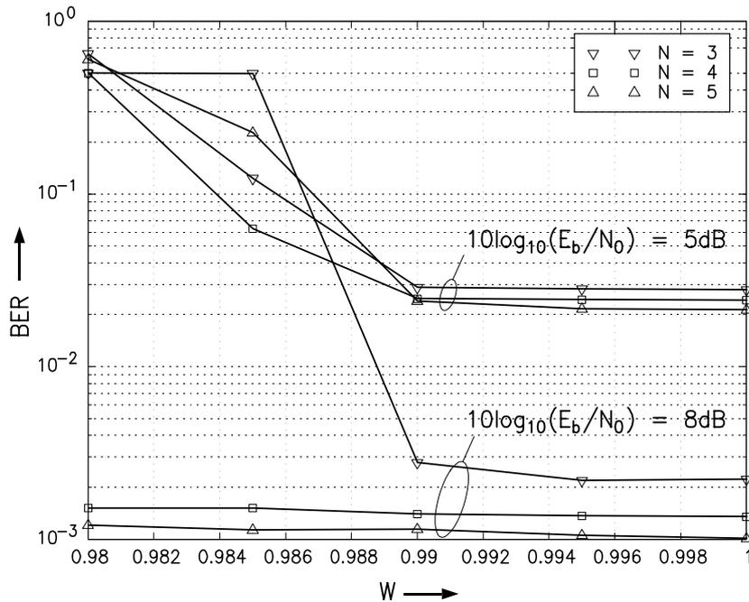
Figure 8: BER vs. forgetting factor  $w$  for the AWGN channel.
