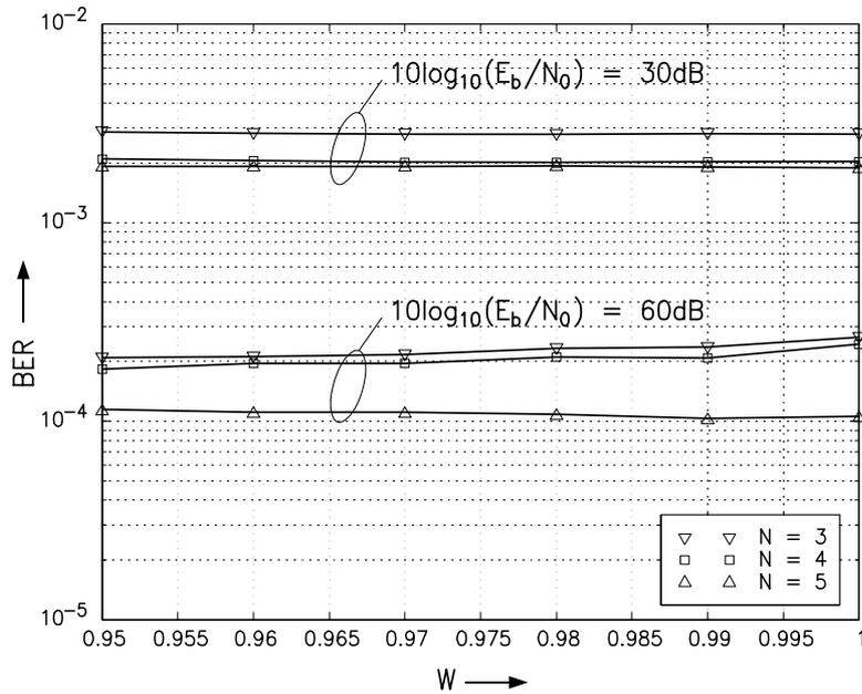
Figure 9: BER vs. forgetting factor  $w$  for the Rayleigh fading channel ( $B_f T = 0.03$ , Jakes model).
