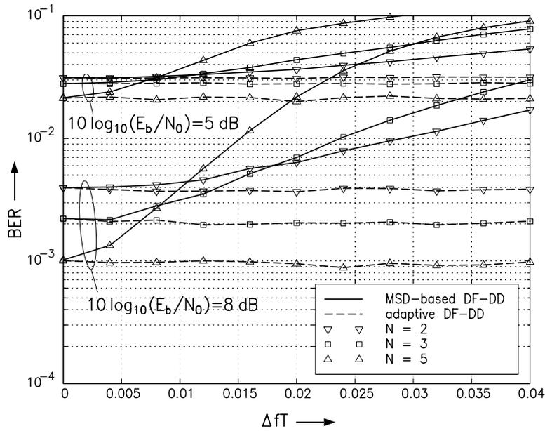
Figure 11: BER vs. normalized frequency offset  $\Delta fT$  for QDPSK with MSD-based DF-DD optimized for AWGN and adaptive (prediction-based) DF-DD ( $w = 1$ ).
