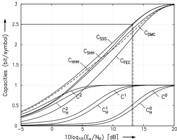
Figure 2: Capacities of 8-ary ASK over the AWGN channel for decoding strategies SSS, SHH, and HHH (see text) and corresponding capacities  $C^i$  and  $C_H^i$  for the equivalent and equivalent binary symmetric channel  $i$ ,  $i = 0, 1, 2$ .
