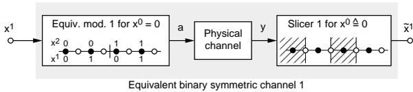
Figure 1: Equivalent BSC 1 for the transmission of symbol  $x^1$  for an 8ASK scheme when hard decision decoding is used and symbol  $x^0 = 0$  is assumed at the lowest level.
