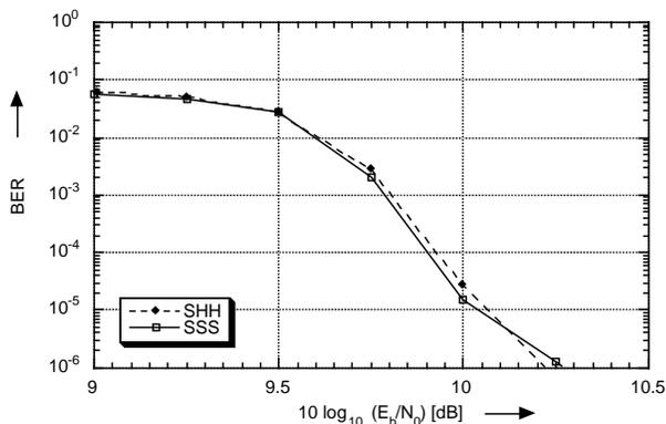
Figure 3: BER of 8ASK transmission with MLC/MSD over the AWGN channel. Code word length  $N = 4095$ . Solid line (case SSS): Rate distribution  $R^0/R^1/R^2 = 0.52/0.98/1.0$ , total rate  $R = 2.5$  bit/symbol. Turbo codes are employed as component codes. Dashed line (case SHH): Rate distribution  $R^0/R^1/R^2 = 0.52/0.96/1.0$ , total rate  $R = 2.48$  bit/symbol. Component codes: Turbo code at level 0, 14-errors-correcting BCH code at level 1. Simulation results.
