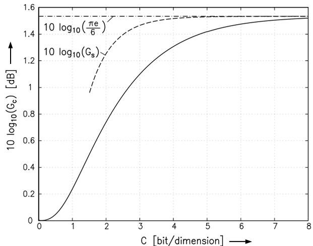
Figure 1: Capacity gain  $G_c$  (solid line) and shaping gain  $G_s$  for discrete constellation (Eq. (1)) (dashed line), resp., vs. capacity.
