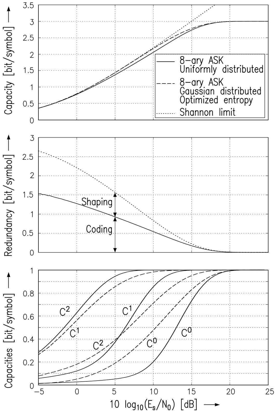
Figure 3: Top: Shannon limit and capacity  $C$  of 8ASK (AWGN channel, Ungerböck's set partitioning) with uniform signaling (solid) and with a optimized discrete Gaussian constellation (dashed). Middle: Sharing of coding and shaping redundancy. Bottom: Capacities  $C^i$  of the equivalent channels of the corresponding MLC scheme.
