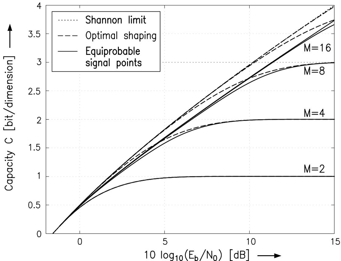
Figure 4: Capacity of ASK schemes with and without shaping.
