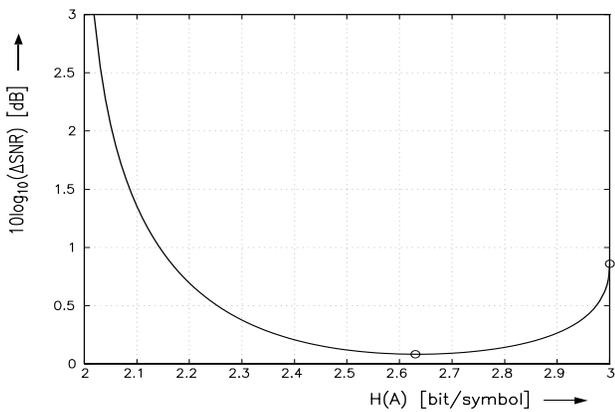
Figure 2: SNR-gap (capacity limit to Shannon limit, see Eq. (3)) for desired rate  $C = 2$  bit/dimension and 8ASK constellation over entropy  $H(A)$  of constellation.
