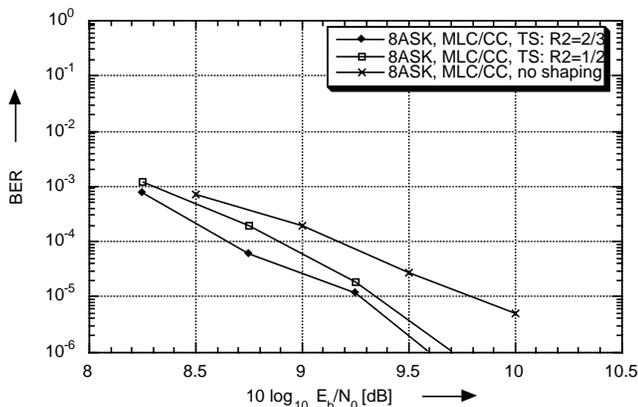
Figure 5: Simulation results: 8ASK with MLC employing (64-state) convolutional codes as components, total rate  $R = 2$  bit/symbol, AWGN channel. Different shaping strategies: 1. Three-dimensional trellis shaping (TS) at highest level ( $R^0/R^1/R^2 = 0.37/0.96/0.67$ ). 2. Two-dimensional TS at highest level ( $R^0/R^1/R^2 = 0.52/0.98/0.5$ ). 3. No shaping is applied ( $R^0/R^1/R^2 = 0.18/0.82/1.0$ ). The desired rates are achieved by puncturing.
