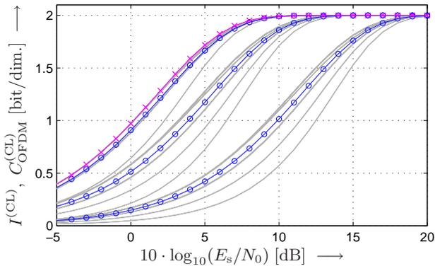
Fig. 2. Individual (gray) and average (with circles) capacities of 4-QAM-OFDM over the AWGN channel (in bits per complex dimension),  $D = 4$ . Left to right: clipping level  $G = 2, 1, .5$ . Crosses: Capacity of unclipped OFDM, equal to the capacity of 4-QAM.
