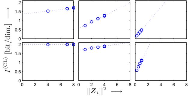
Fig. 3. Scatter plots of the individual capacities  $I^{(\text{CL})}(\mathbf{A}_i; \mathbf{Y})$  versus the energy  $\|\mathbf{Z}_i\|^2$  of the OFDM frame after clipping,  $D = 4$ . Top row:  $E_s/N_0 \hat{=} 5$  dB, bottom row:  $E_s/N_0 \hat{=} 10$  dB. Left to right: clipping level  $G = 2, 1, .5$ . Dotted: straight-line fit.
