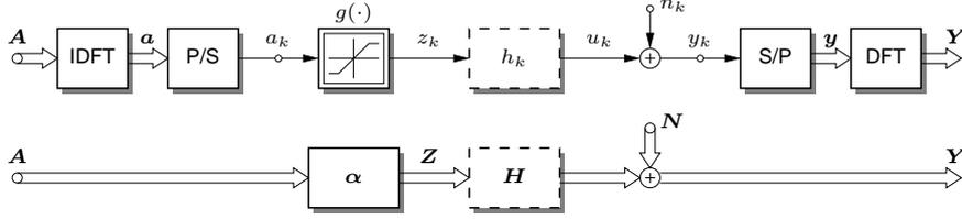
Fig. 1. OFDM system model with nonlinear operation on the transmit symbols. Top: time-domain description; bottom: frequency-domain model.
