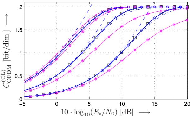
Fig. 5. Average capacities of 4-QAM-OFDM over the AWGN channel (circles) together with the Shannon (dashed) and the QAM (squares) upper bounds, the lower bound (dash-dotted), and the statistical model (stars) for  $G = 2, 1, .5$ .  $D = 4$ . Crosses: Capacity of unclipped OFDM, equal to the capacity of 4-QAM.
