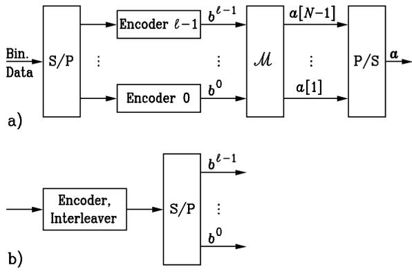
Figure 3: Channel encoding and Mapping: a) MLC, b) Changes for BICM.
