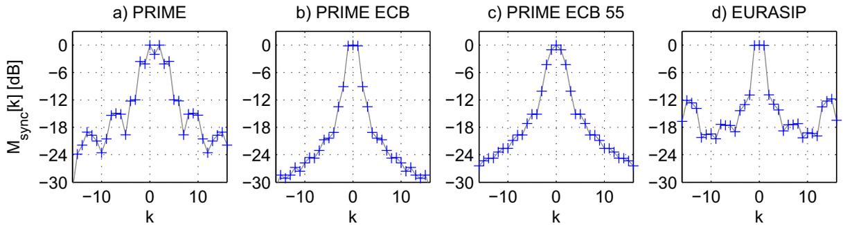
Fig. 6. Synchronization Metric with  $L = 3$  in Noise- and Distortion-Free Environment for Various Preambles: “PRIME” – Preamble  $p[n]$ , “PRIME ECB” – Preamble  $p_{\text{ECB}}[n]$ , “PRIME ECB 55” – Part of 55 Samples of  $p_{\text{ECB}}[n]$ , “EURASIP” – Preamble of [4].
