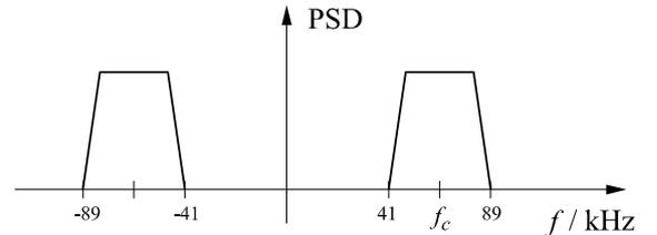
Fig. 1. Typical PSD of PRIME
