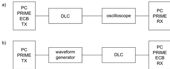
Fig. 7. Trial Setup: a) Transmission DLC to PRIME, b) PRIME to DLC
