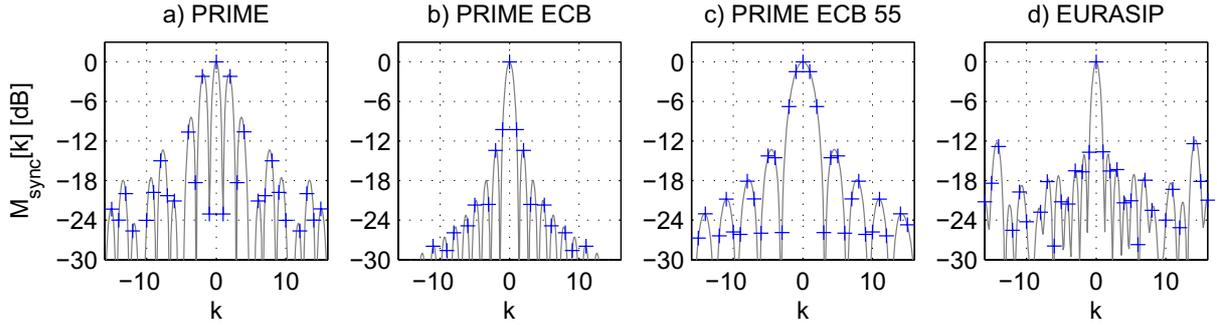
Fig. 5. Synchronization Metric with  $L = 1$  in Noise- and Distortion-Free Environment for Various Preambles: “PRIME” – Preamble  $p[n]$ , “PRIME ECB” – Preamble  $p_{\text{ECB}}[n]$ , “PRIME ECB 55” – Part of 55 Samples of  $p_{\text{ECB}}[n]$ , “EURASIP” – Preamble of [4].
