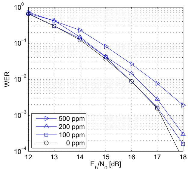
Fig. 4. Word Error Rate for Different Sampling Frequency Offsets
