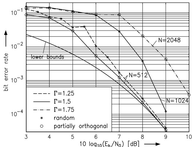
Fig. 1: Bit error rate of ISDIC-OSC [2] vs. signal-to-noise ratio by means of simulation and compared to the lower bound<sup>1</sup>
