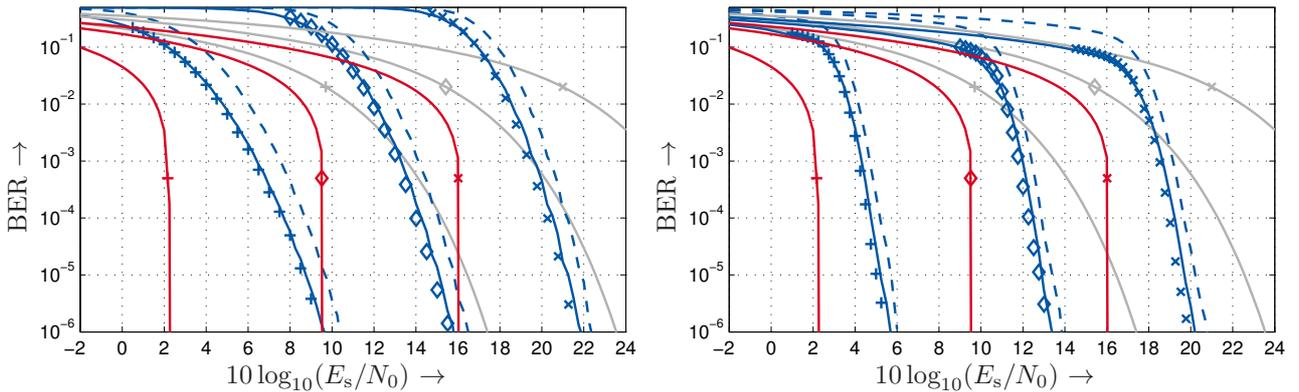
Fig. 5. BER estimates (solid/dashed: lower/upper bound) for Gray-labeled BICM-ASK (blue, left-to-right: 4- (+), 8- ( $\diamond$ ), 16-ASK ( $\times$ )) using convolutional codes ( $\nu = 4$ ) with soft-input Viterbi decoding (left) and LDPC codes with soft-input belief-propagation decoding (right). For comparison: Simulation results of BICM-ASK with corresponding coding scheme (markers), ideal coding scheme/rate-distortion capacity bound (red), uncoded transmission (gray).
