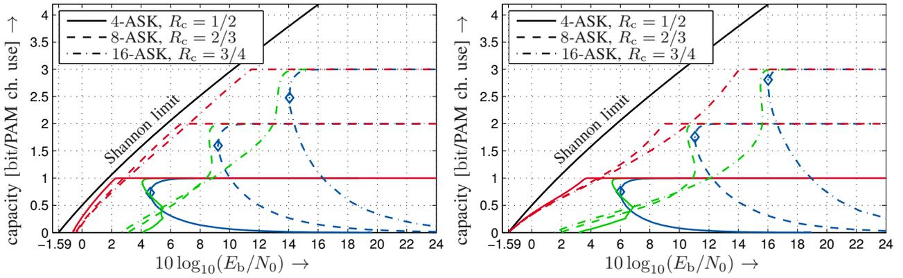
Fig. 7. Capacity estimates for BICM-ASK (left: Gray-labeling, right: set-partition labeling) using convolutional codes ( $\nu = 4$ ) with soft-input Viterbi decoding (blue) and LDPC codes with soft-input BP decoding (green) plotted vs.  $E_b/N_0$ . For comparison: Ideal coding scheme (red).
