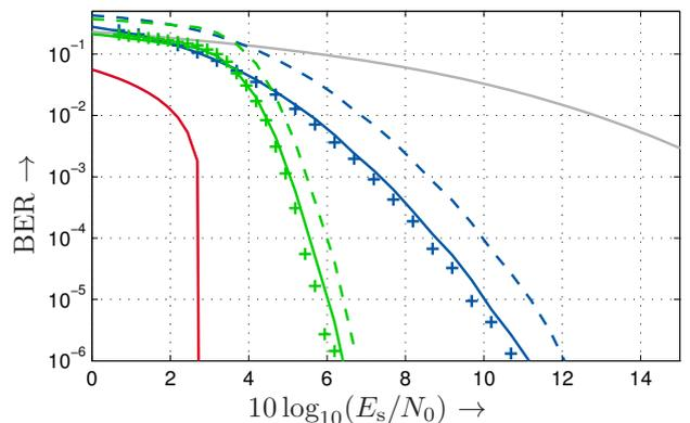
Fig. 6. BER estimates compared to simulation results for 4-ASK using a convolutional code ( $R_c = 1/2$ ,  $\nu = 4$ ) with soft-input Viterbi-decoding (blue), an LDPC code ( $R_c = 1/2$ , codeword length  $n = 648$ ) with BP decoding (green), and uncoded transmission (gray) subject to log-normal fading.
