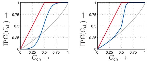
Fig. 2. IPCs of rate-1/2 coding schemes. Left: convolutional code (nonsystematic encoding, constraint length  $\nu = 4$ ) with soft-input Viterbi decoding. Right: LDPC code (from WLAN-802.11n std., systematic encoding, codeword length 648) with BP decoding. Red: ideal coding scheme. Gray: uncoded.
