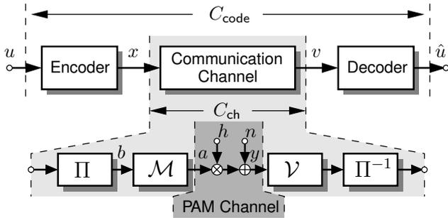
Fig. 1. System model of coded transmission. Top: generic model, bottom: BICM-ASK for the communication channel.
