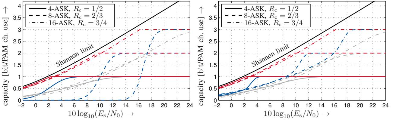
Fig. 4. Capacity estimates for Gray-labeled BICM-ASK (blue) using convolutional codes ( $\nu = 4$ ) with soft-input Viterbi decoding (left) and LDPC codes with soft-input belief-propagation decoding (right). For comparison: Ideal coding scheme (red), uncoded transmission (gray, scaled by  $R_c$ ).
