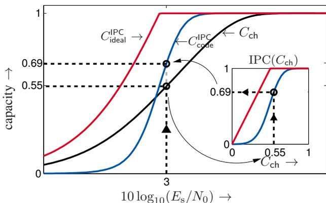
Fig. 3. Illustration of IPC-based estimation of the capacity of the end-to-end coded channel for BICM using Gray-labeled 4-ASK with the convolutional code and soft-input Viterbi decoding shown in Fig. 2 (left).
