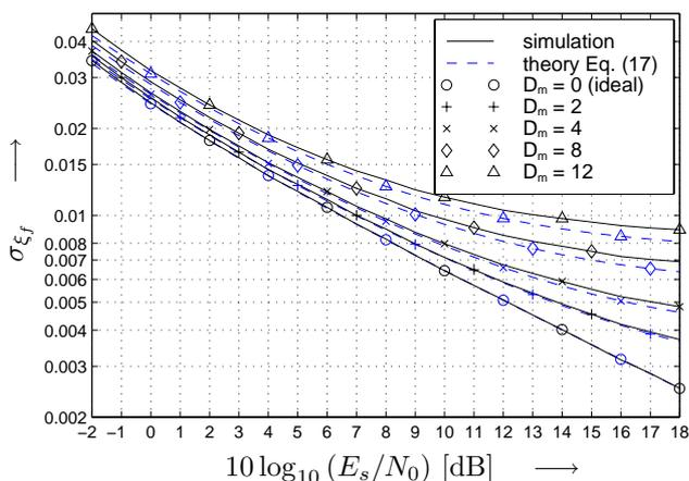
Figure 5: Simulation results and prediction from (17) for the NFO stdv  $\sigma_{\xi_f}$  over SNR with some fixed frame misplacement  $D_m$  as parameter.
