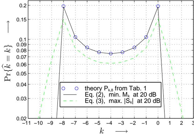
Figure 4: Simulated lock-in probabilities obtained with criteria in Eqs. (2) and (3) in a non-dispersive channel at  $10 \log_{10}(E_s/N_0) = 20$  dB. The theoretical results for the conditional lock-in probabilities  $P_{k,8}$  are plotted for comparison (cf. Tab. 1).
