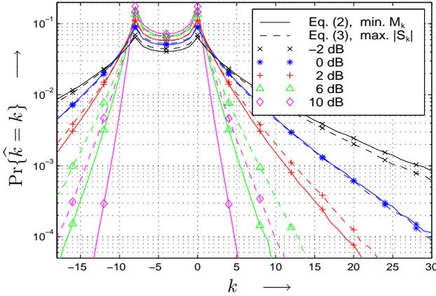
Figure 2: Simulated lock-in histogram in a non-dispersive channel at various  $10 \log_{10}(E_s/N_0)$  [dB]. The frame sync. criteria in Eqs. (2) and (3) are compared. The parameters are  $D_s = D = 64$  and  $D_g = 8$ .
