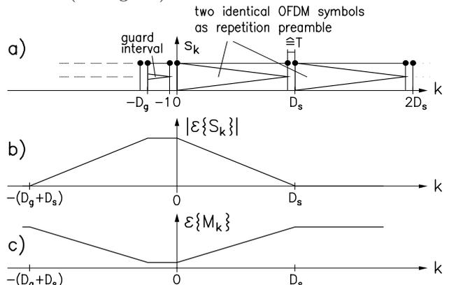
Figure 1: Symbolical illustration of the repetition preamble together with the expected values ( $\mathcal{E}\{\cdot\}$ ) of the frame synchronization metrics  $M_k$  and  $S_k$ .
