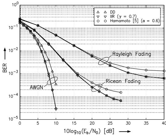
Figure 6: BER of QDPSK ( $M = 4$ ) vs.  $E_b/N_0$  for DD, noise prediction with IIR filter, and the scheme proposed in [4, 5] for AWGN, Rayleigh fading ( $f_d T = 0.0075$ ), and Ricean fading ( $R = 7$  dB,  $f_d T = 0.03$ ) channels.
