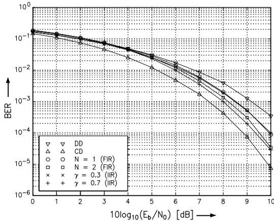
Figure 5: BER of QDPSK ( $M = 4$ ) vs.  $E_b/N_0$  for DD, CD, and noise prediction with FIR and IIR filter under AWGN conditions.
