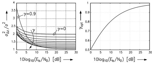
Figure 4: a) Normalized variance  $\frac{\sigma_{\Delta z}^2}{\sigma^2}$  vs.  $E_b/N_0$  for QDPSK;  $\gamma$  varies from 0 to 0.9 in steps of 0.1; b) optimum filter coefficient  $\gamma_{\text{opt}}$  vs.  $E_b/N_0$  for QDPSK.
