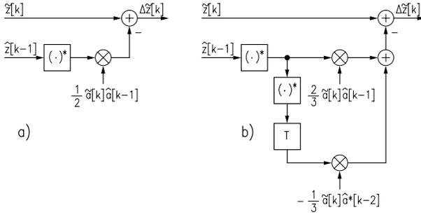
Figure 2: Noise prediction using an FIR filter: a)  $N = 1$ ; b)  $N = 2$ .
