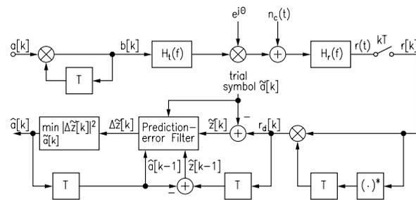
Figure 1: Block diagram of the transmission model for AWGN channel and constant phase shift  $\Theta$ .
