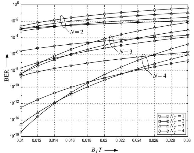
Figure 2: BER vs.  $B_f T$  for DF-DD.  $R = 2 \text{ bits}/(\text{channel use})$ ,  $\text{SNR} \rightarrow \infty$ , and  $N_R = 1$  are valid.
