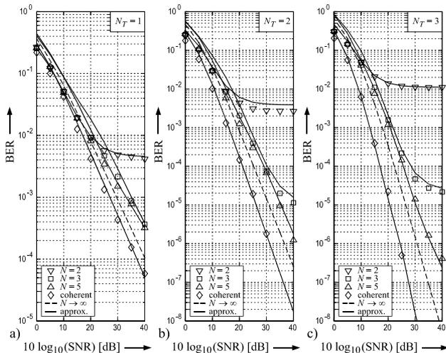
Figure 1: BER vs.  $10 \log_{10}(\text{SNR})$  for DF-DD with a)  $N_T = 1$ , b)  $N_T = 2$ , and c)  $N_T = 3$  transmit antennas.  $\nabla$ ,  $\square$ ,  $\triangle$ , and  $\diamond$  denote simulation points.  $R = 1 \text{ bit}/(\text{channel use})$ ,  $B_f T = 0.03$ , and  $N_R = 1$  are valid.
