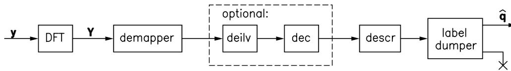
Fig. 3. SLM-OFDM receiver for scrambling approach. No explicit side information is required.
