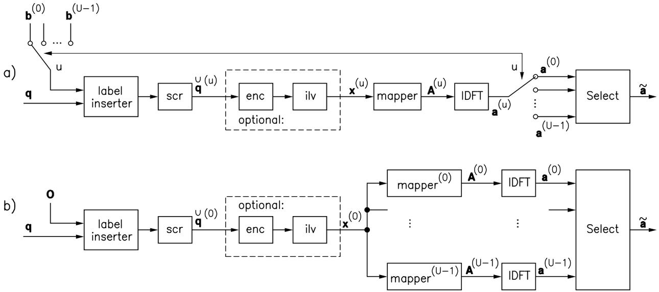
Fig. 1. SLM-OFDM transmitter with label insertion and scrambling approach.
