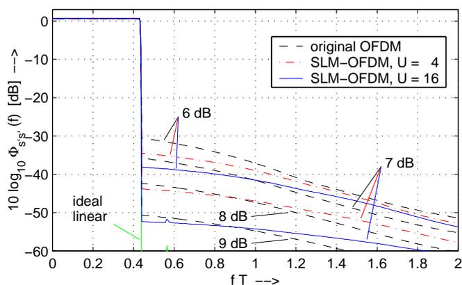
Fig. 7. Power spectral density of  $s'(t)$  after ideally linear and soft-limiting nonlinear characteristic for original OFDM and SLM-OFDM for various back-offs.
