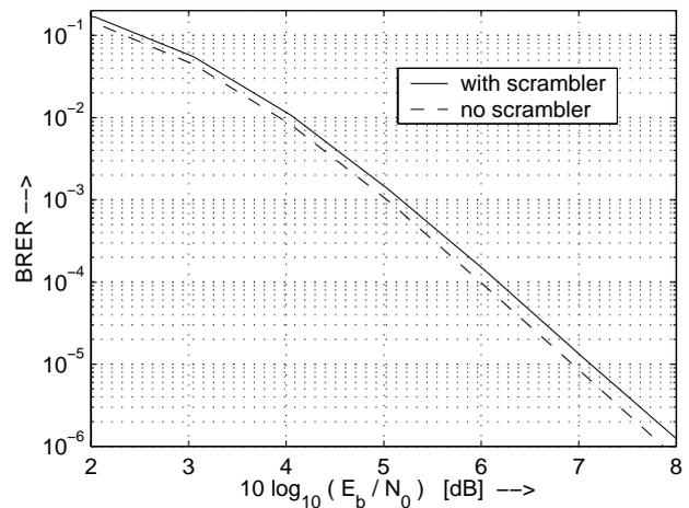
Fig. 6. Bit residual error rate in AWGN, i.e., after convolutional decoding for original OFDM and scrambled SLM-OFDM.
