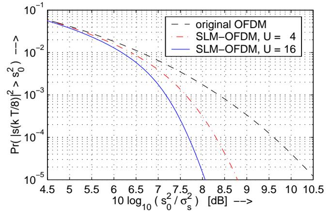
Fig. 5. Power-excess probability for transmit signal  $s(t)$ .
