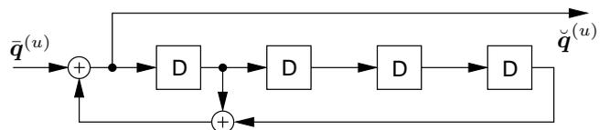
Fig. 2. Scrambler of memory 4 with feedback polynomial  $1+x+x^4$ .
