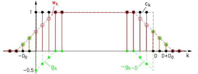
Fig. 1. Exemplary decomposition [7] of a trapezoidal Nyquist receiver time window  $w_k$  into the sum of a rectangular (i.e.,  $c_k$ ) and two rolloff modifications (i.e.,  $g_k$  and  $-g_{k-D}$ ) with  $D_\theta = 2$ .
