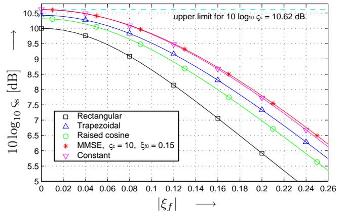
Fig. 3. Subcarrier SNR vs. NFO for various Nyquist rolloff shapes with  $D_\theta = 8$  at  $D = 64$ , i.e.,  $\theta = 0.266$ . The channel SNR is  $10 \log_{10} \zeta_c = 10$  dB.
