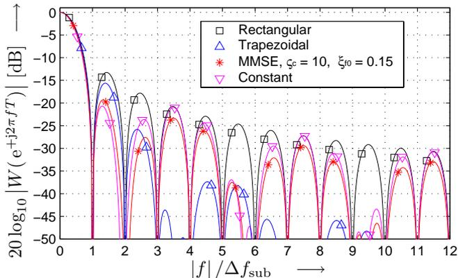
Fig. 4. Effective frequency responses for subcarrier demodulation with four different receiver window shapes with  $D_\theta = 8$  and  $D = 64$ , i.e.,  $\theta = 0.266$ .
