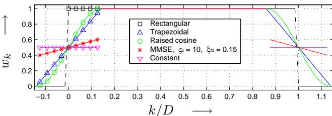
Fig. 2. Various Nyquist rolloff shapes  $\mathbf{w}$  with  $D_\theta = 8$  and  $D = 64$  so that the window has a time-excess factor of  $\theta = 0.266$ . The conventional rectangular window is dashed with  $\square$  marks.
