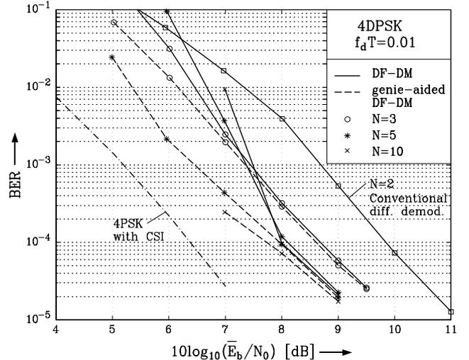
Figure 5: BER versus  $10 \log_{10}(\bar{E}_b/N_0)$  for 4DPSK and Rayleigh fading with  $f_d T = 0.01$ . 64 states convolutional code. DF-DM with four iterations. Solid lines: conventional differential demodulation with  $N = 2$  and DF-DM with  $N = 3, 5, 10$ . Dashed lines: genie-aided DF-DM. Dash-dotted line: 4PSK with perfect CSI.
