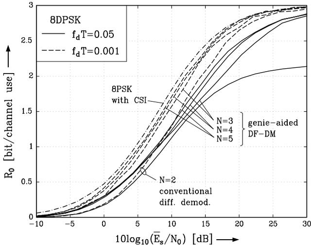
Figure 4: Cutoff rate for 8DPSK and Rayleigh fading. Conventional differential demodulation with  $N = 2$  and genie-aided DF-DM with  $N = 3, 4, 5$ . Dashed lines:  $f_d T = 0.001$ . Solid lines:  $f_d T = 0.05$ . Dash-dotted line: 8PSK with perfect CSI.
