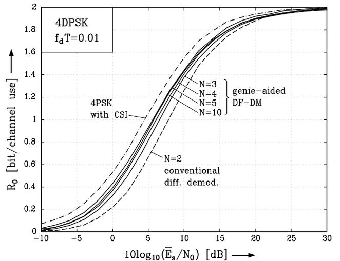
Figure 3: Cutoff rate for 4DPSK and Rayleigh fading with  $f_d T = 0.01$ . Dashed line: conventional differential demodulation with  $N = 2$ . Solid lines: genie-aided DF-DM with  $N = 3, 4, 5, 10$ . Dash-dotted line: 4PSK with perfect CSI.
