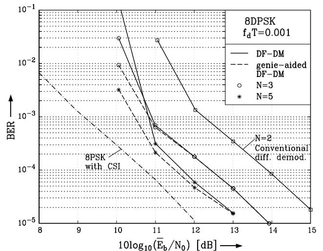
Figure 7: BER versus  $10 \log_{10}(\bar{E}_b/N_0)$  for 8DPSK and Rayleigh fading with  $f_d T = 0.001$ . 64 states convolutional code. DF-DM with four iterations. Solid lines: conventional differential demodulation with  $N = 2$  and DF-DM with  $N = 3, 5$ . Dashed lines: genie-aided DF-DM. Dash-dotted line: 8PSK with perfect CSI.
