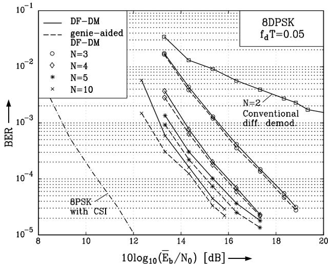
Figure 6: BER versus  $10 \log_{10}(\bar{E}_b/N_0)$  for 8DPSK and Rayleigh fading with  $f_d T = 0.05$ . 64 states convolutional code. DF-DM with four iterations. Solid lines: conventional differential demodulation with  $N = 2$  and DF-DM with  $N = 3, 4, 5, 10$ . Dashed lines: genie-aided DF-DM. Dash-dotted line: 8PSK with perfect CSI.
