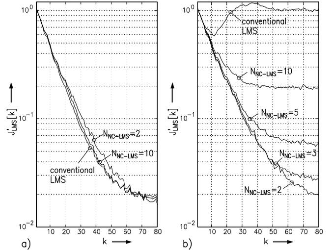
Figure 2: Learning curves for NC-LMS and conventional LMS algorithm with a)  $\Delta f T = 0$ , and b)  $\Delta f T = 0.02$ . For both figures  $10 \log_{10}(E_b/N_0) = 15$  dB and  $\delta_{\text{LMS}} = 0.05$  are valid.
