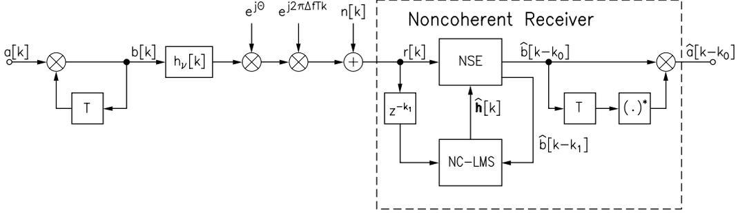
Figure 1: Block diagram of the discrete-time transmission and receiver model under consideration.
