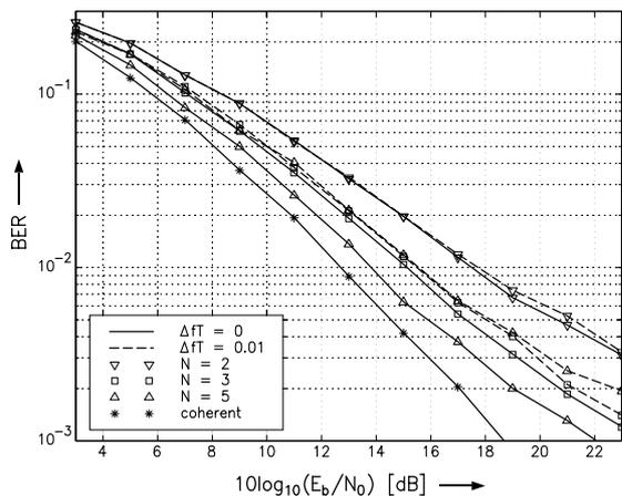
Figure 3: BER vs.  $10 \log_{10}(E_b/N_0)$  for NSE combined with the NC-LMS algorithm and coherent MLSE combined with the conventional LMS algorithm. A three-tap Rayleigh fading channel is used.
