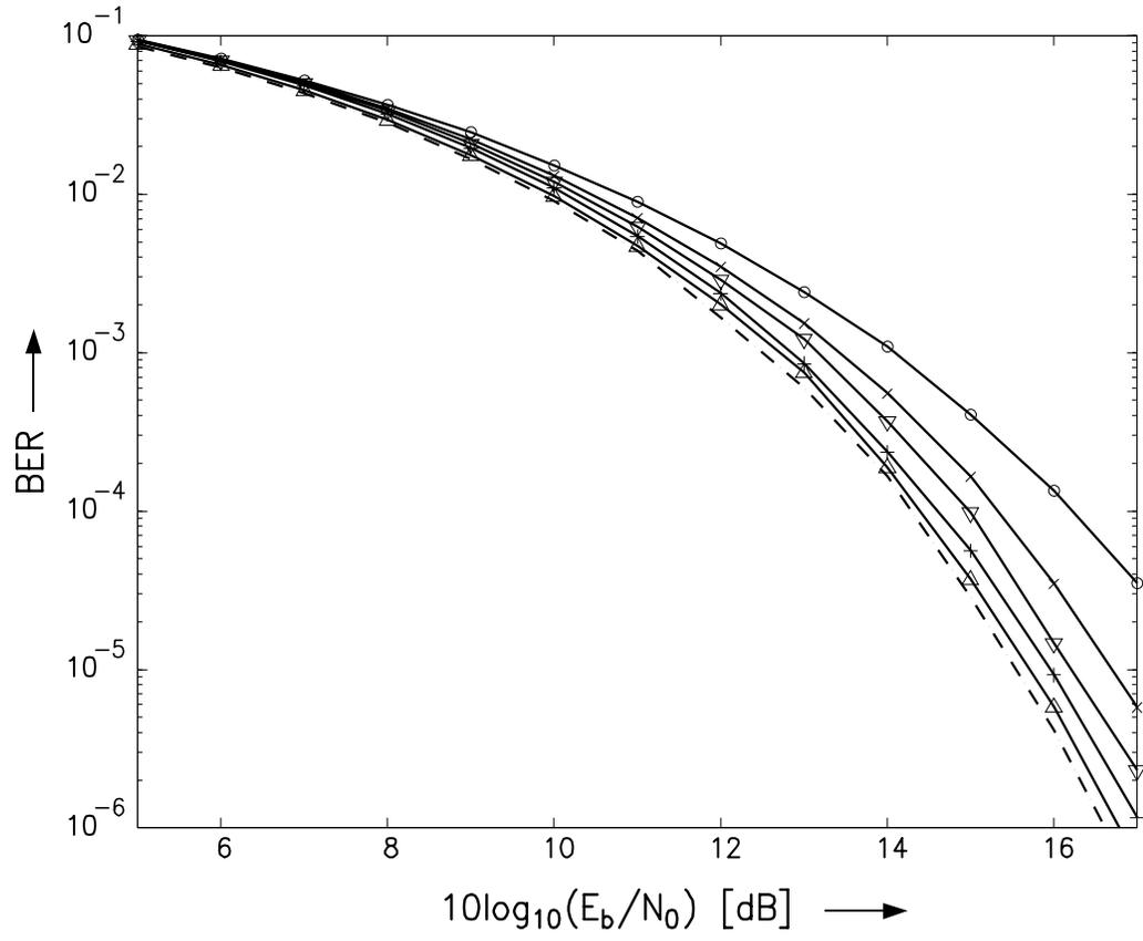
Figure 2: Error performance of the proposed DF-DD scheme with recursively generated symbol  $\hat{r}[k-1]$  according to eqn. 7.
