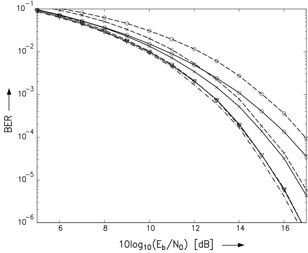
Figure 1: Comparison of the proposed DF-DD scheme with nonrecursively generated symbol  $\tilde{r}[k-1]$  according to eqn. 4 and the scheme of [2].
