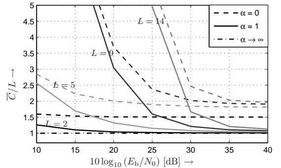
Fig. 3. Average complexity  $\bar{C}/L$  over SNR for the SD with stopping radius ( $\alpha = 1$ ) and without stopping radius ( $\alpha = 0$ ) for different  $L$ . DF-DD benchmark is also included ( $\alpha \rightarrow \infty$ ).
