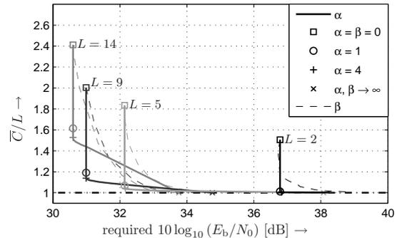
Fig. 4. Average complexity  $\bar{C}/L$  of the SD with scaled stopping radius over SNR required to achieve  $\text{BER} = 5 \cdot 10^{-4}$ , for  $M = 4$ ,  $B_f T = 0.01$ , and different  $L$ . Curves for a fixed  $R_{\text{stop}}^2 = \beta \cdot L$  (dashed lines, cf. [7]) are also included for a comparison.
