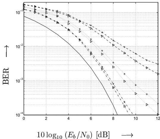
Figure 1: BER vs.  $10 \log_{10}(E_b/N_0)$  for  $\beta = 0.75$  (---),  $\beta = 1$  (···) and  $\beta = 1.25$  (-·-) for ISDIC1 (+), ISDIC2 ( $\triangleright$ ), and SUB (-).
