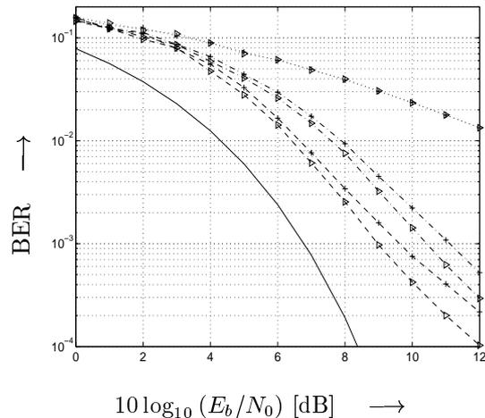
Figure 2: BER vs.  $10 \log_{10}(E_b/N_0)$  for  $\beta = 1$  after 1st iteration (···), 2nd iteration (-·-), and 4th iteration (---) for ISDIC1 (+), ISDIC2 ( $\triangleright$ ) and SUB (-).
