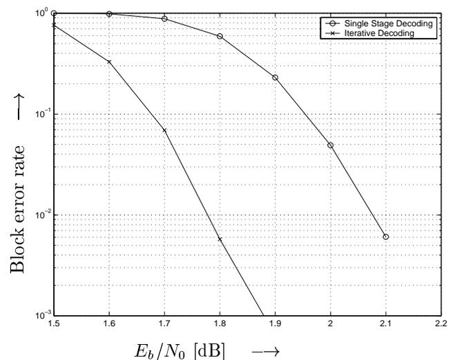
Figure 2: Performance of the ESA Telemetry Codes with soft–out BCJR–Decoding and Error and Erasure RS–Decoding.
