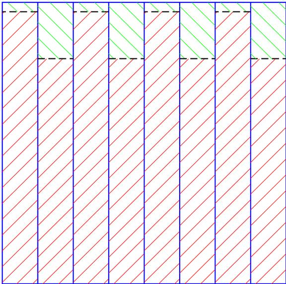
Figure 3: Interleaving for a hierarchically concatenated coding scheme (RS-codewords vertically, upper part is redundancy, lower part information).
