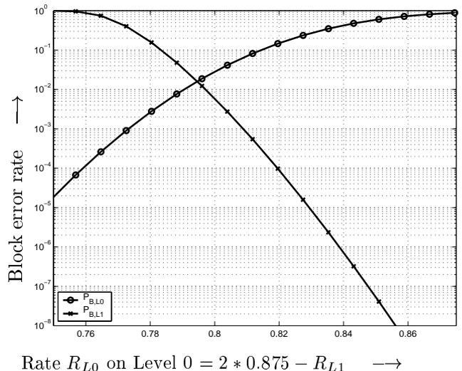
Figure 6: Plot of error rates for both levels for  $E_b/N_0 = 2.2dB$ .
