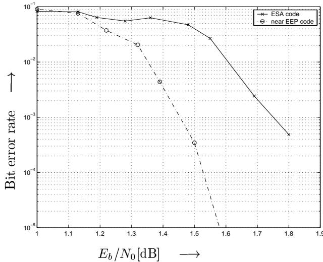
Figure 7: Performance-comparison of the EEP and hierarchical near-EEP code-concatenation.
