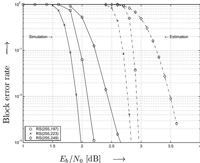
Figure 4: Comparison of Estimation and Simulation of the concatenation of RS(255,197), RS(255,223) and RS(255,249) with a inner convolutional code using Viterbi-decoding of the inner code.
