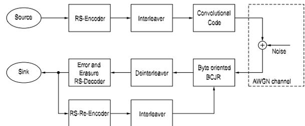
Figure 1: Blockdiagram of a Transmission scheme with the ESA telemetry code.
