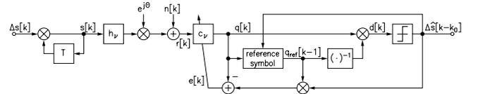
Figure 1: Block diagram of the discrete-time transmission model with NMIE.
