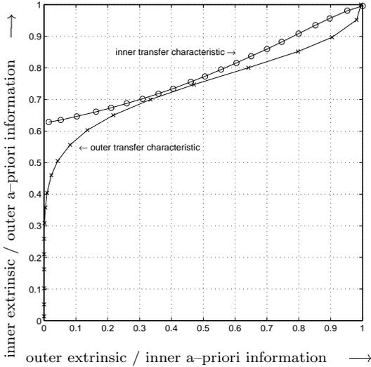
Figure 3: EXIT-Chart for a classical woven convolutional code at  $E_b/\mathcal{N}_0 = 0.8$  dB ( $m = 2$ ,  $R_i = 2/3$ ,  $R_o = 3/4$ ).
