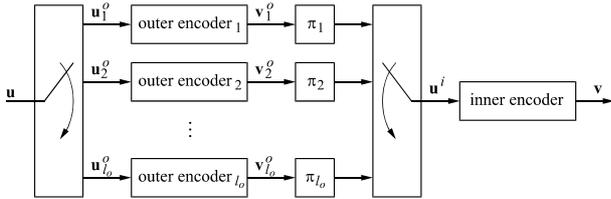
Figure 1: Woven convolutional code : *outer warp* with *row wise* interleaving.
