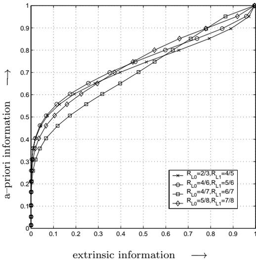
Figure 4: Transfer characteristics of hierarchically constructed outer codes.
