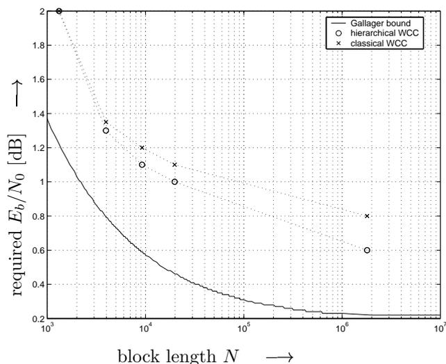
Figure 6: Spectral efficiency of Woven Convolutional Codes.
