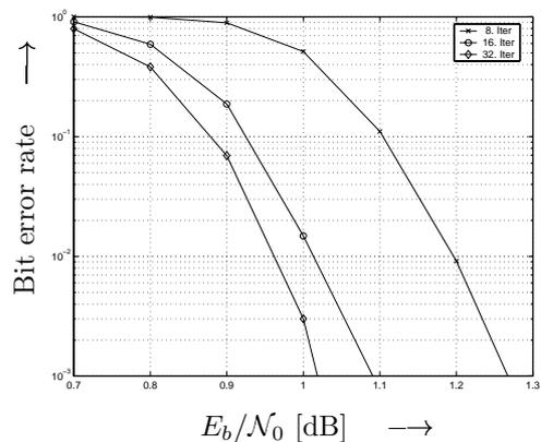
Figure 2: Performance of a classical woven convolutional code ( $m = 2$ ,  $R_i = 2/3$ ,  $R_o = 3/4$ ,  $K = 9900$ ,  $N = 19800$ ,  $l_o = 10$ ).
