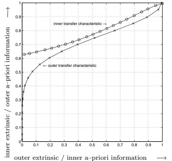
Figure 5: EXIT-Chart for a hierarchical woven convolutional code at  $E_b/\mathcal{N}_0 = 0.8$  dB ( $m = 2$ ,  $R_i = 2/3$ ,  $R_{L0} = 2/3$ ,  $R_{L1} = 4/5$ ).
