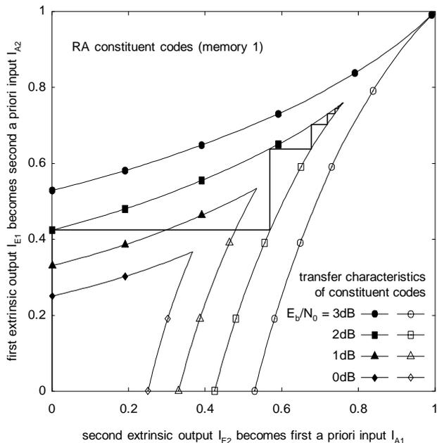
Figure 6: Extrinsic Information Transfer (EXIT) Chart for parallel representation of RA-Codes.
