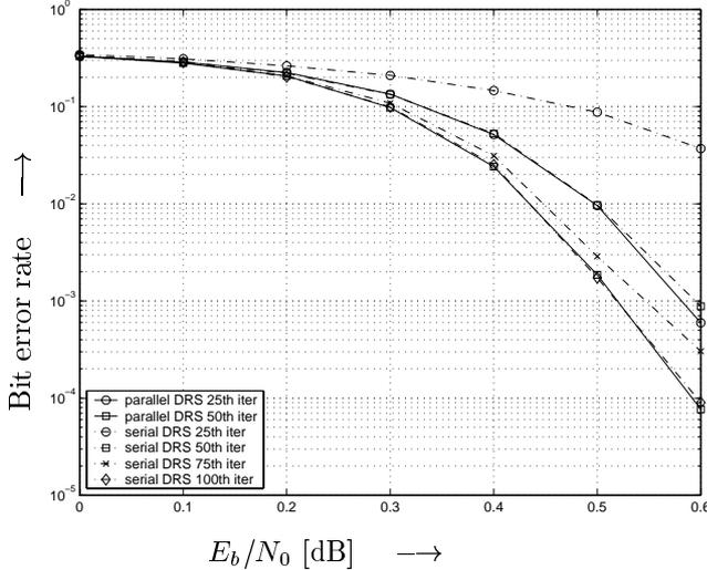
Figure 13: Performance of the rate  $R = 1/2$  DRS-Code in serial and parallel representation in dependence of number of iteration (Blocklength  $K = 10000$ ).
