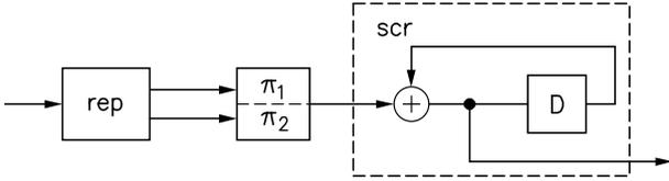
Figure 2: RA-Code with splitted interleaver.
