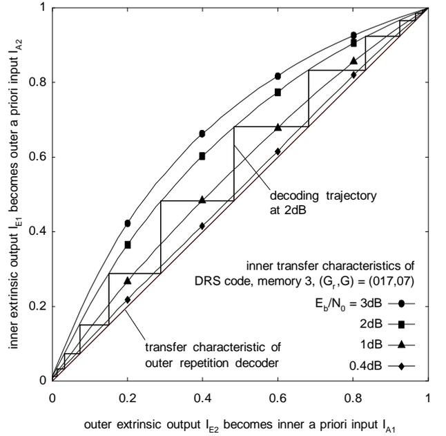
Figure 11: Extrinsic Information Transfer (EXIT) Chart for serial representation of the DRS-Code.
