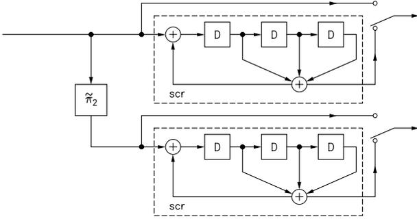
Figure 9: Rate  $R = 1/2$  DRS-Code with splitted interleaver and separated scramblers.
