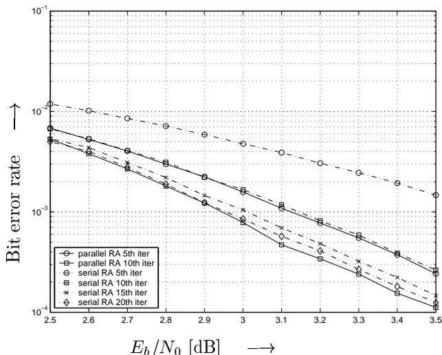
Figure 7: Performance of RA-Codes in serial and parallel representation in dependence of number of iteration (Blocklength  $K = 10000$ ).
