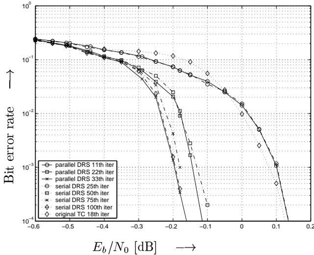
Figure 16: Performance of the rate  $R = 1/3$  DRS-Code in serial and parallel representation in dependence of number of iteration (Blocklength  $K = 10000$ ). For comparison the performance of the original  $R = 1/3$  Turbo-Code [3] for  $K = 10000$  and 18 Iterationen is also given.
