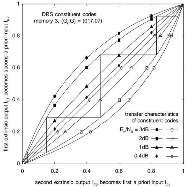
Figure 12: Extrinsic Information Transfer (EXIT) Chart for parallel representation of the DRS-Code.
