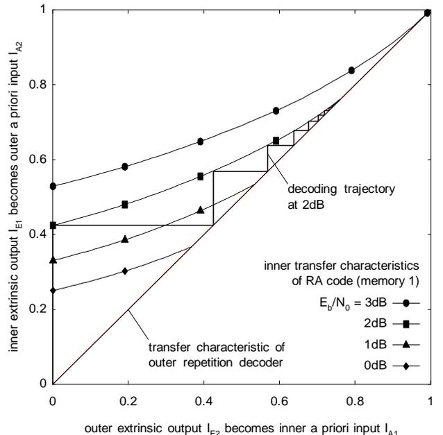
Figure 5: Extrinsic Information Transfer (EXIT) Chart for serial representation of RA-Codes.
