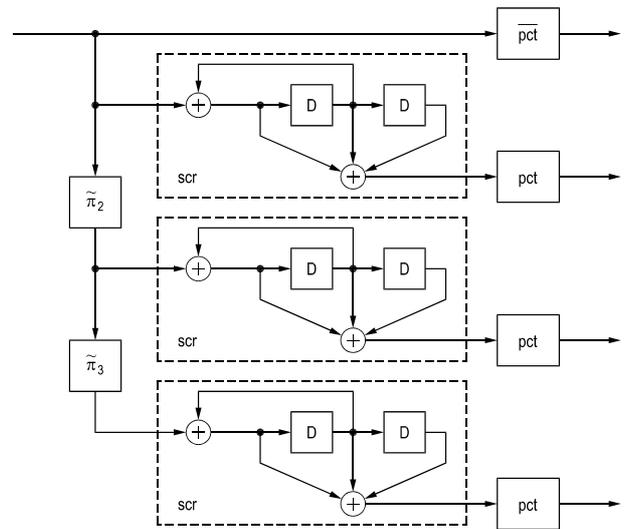
Figure 15: Turbo-Code representation of rate  $R = 1/3$  DRS-Codes.
