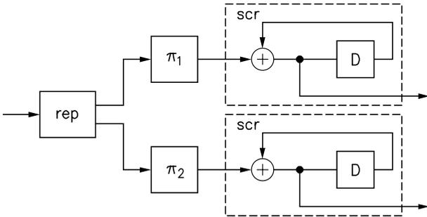
Figure 3: RA-Code with splitted interleaver and separated scramblers.
