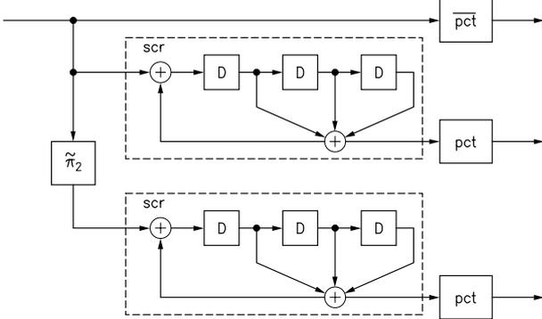
Figure 10: Turbo-Code representation of rate  $R = 1/2$  DRS-Codes.
