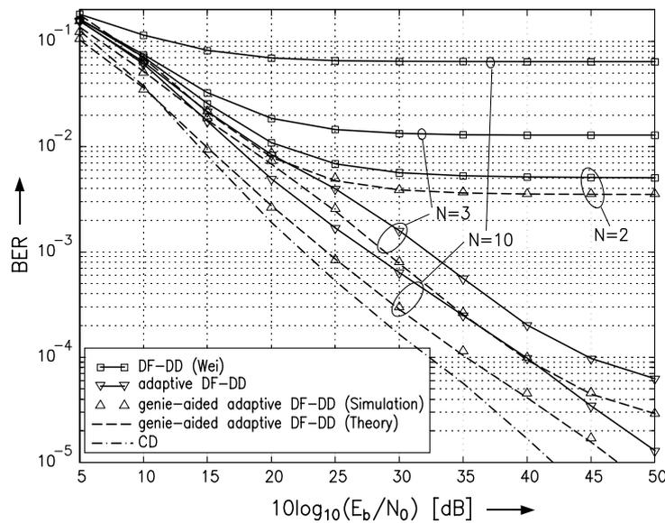
Figure 3: BER vs.  $10 \log_{10}(E_b/N_0)$  for DF-DD proposed by Wei et al., adaptive DF-DD, genie-aided adaptive DF-DD (simulation and theory), and CD for a Ricean fading channel ( $10 \log_{10}(K) = 5$  dB,  $f_D T = 0.015$ ,  $B_f T = 0.03$ ,  $a_0 = 2.0$ ).
