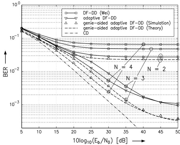
Figure 2: BER vs.  $10 \log_{10}(E_b/N_0)$  for DF-DD proposed by Wei et al., adaptive DF-DD, genie-aided adaptive DF-DD (simulation and theory), and CD for a Rayleigh fading channel ( $B_f T = 0.03$ ,  $a_0 = 2.0$ ).
