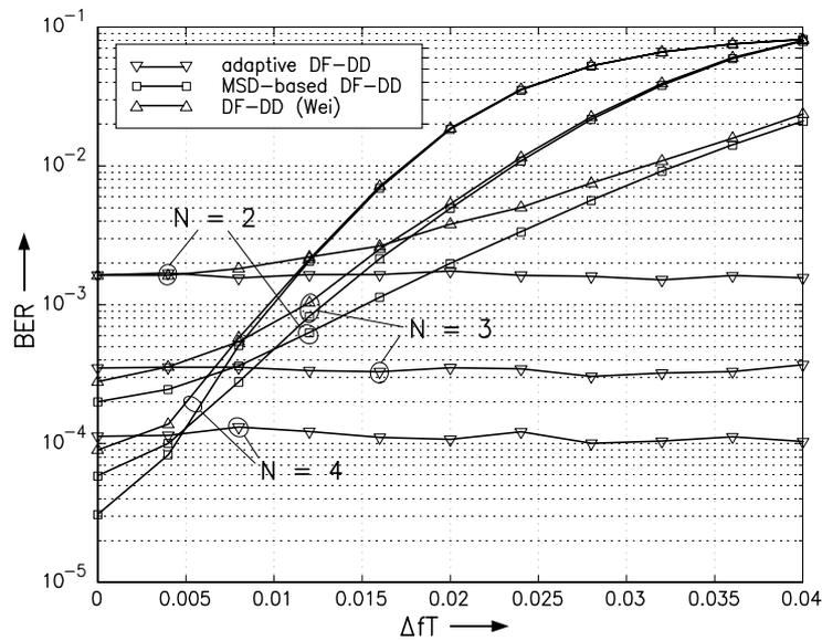
Figure 1: BER vs.  $\Delta fT$  for DF-DD proposed by Wei et al., MSD-based DF-DD, and adaptive DF-DD.  $10 \log_{10}(E_b/N_0) = 15$  dB and  $a_0 = 1.8$  are valid.
