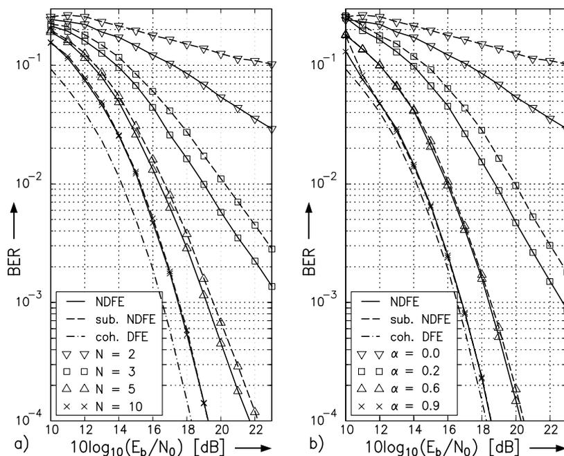
Figure 7: BER vs.  $10 \log_{10}(E_b/N_0)$  for NDFE and suboptimum NDFE with a) nonrecursively and b) recursively generated phase reference symbol. Channel B is used and for comparison the BER for coherent MMSE-DFE is also shown.
