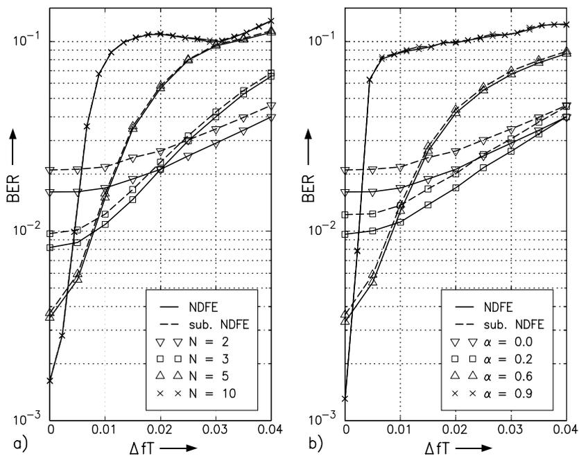
Figure 8: BER vs.  $\Delta fT$  for NDFE and suboptimum NDFE with a) nonrecursively and b) recursively generated phase reference symbol.
