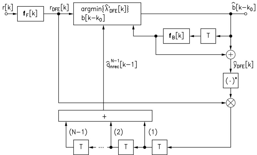
Figure 2: Receiver structure for the proposed NDFE scheme.
