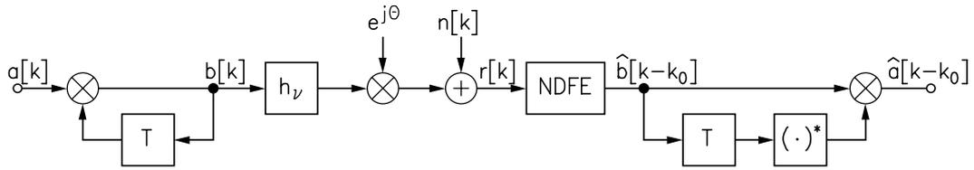
Figure 1: Block diagram of the discrete-time transmission model under consideration.
