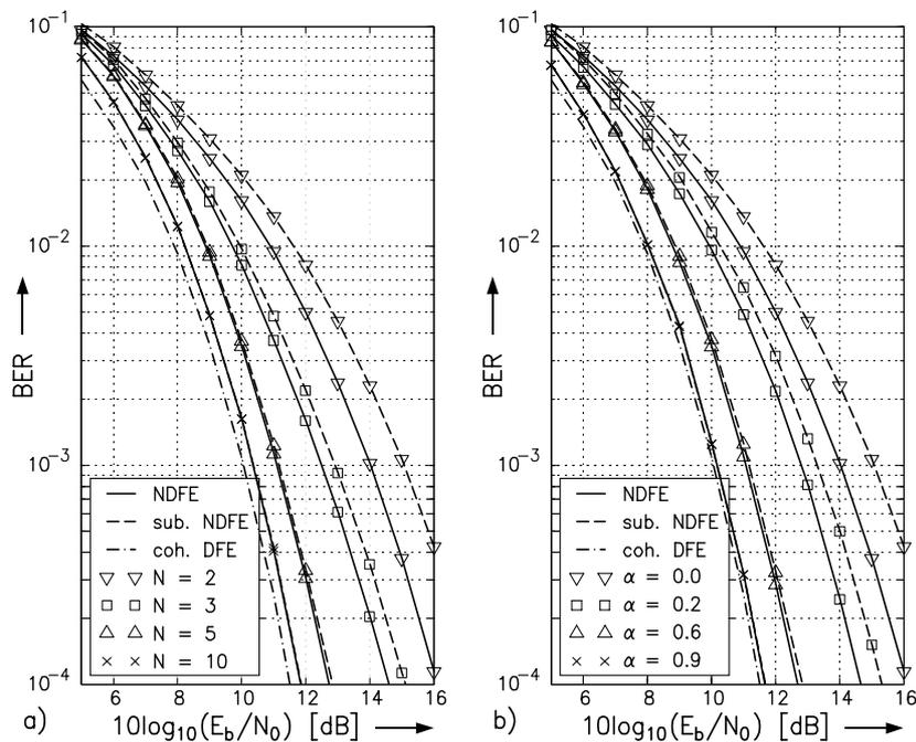
Figure 6: BER vs.  $10 \log_{10}(E_b/N_0)$  for NDFE and suboptimum NDFE with a) non-recursively and b) recursively generated phase reference symbol. Channel A is used and for comparison the BER for coherent MMSE-DFE is also shown.
