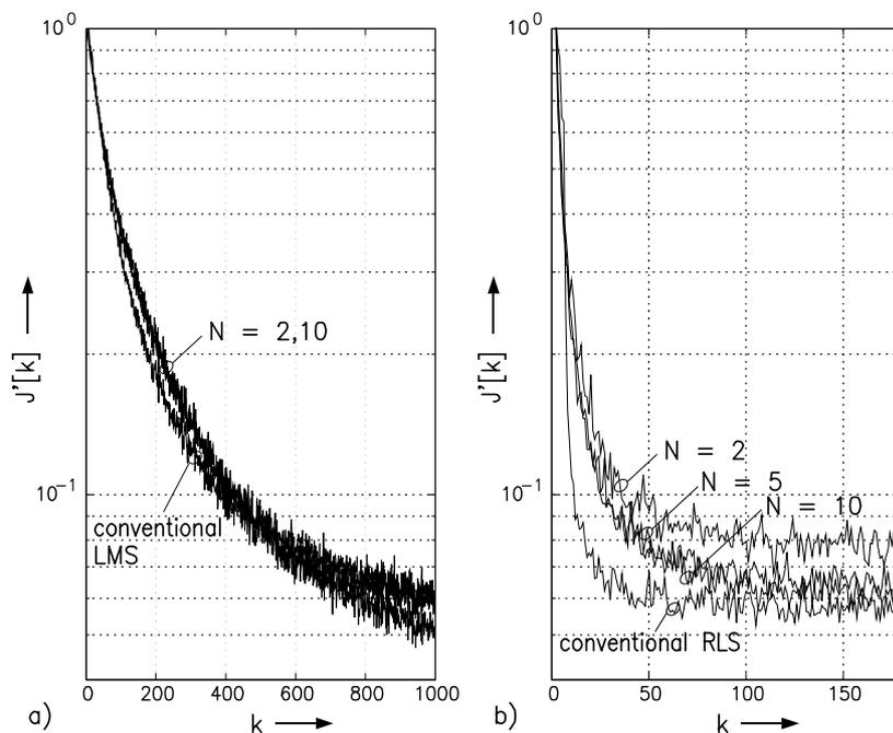
Figure 4: Learning curves for a) modified and conventional LMS algorithm; b) modified and conventional RLS algorithm.
